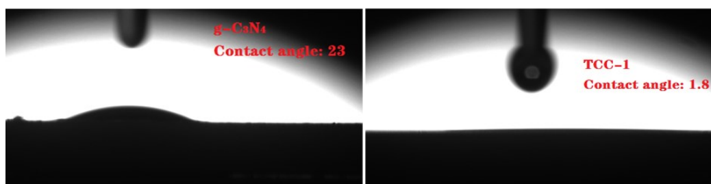
S-Fig. 3. Contact angle measurements of water drop on the surface of the thin films of g-C 3 N 4 and TCC-1.
