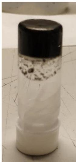
**Figure S1** Photograph of the final viscous stable graphene ink (upside down).
