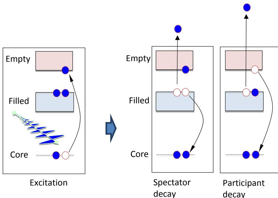
**Figure S5.** Schematic energy level diagram in Resonant photoemission. a) schematics of core electron excitation to empty state, followed by b) decay of the core hole in which the excited electron spectates the emission of Auger electron and c) core hole decay in which the excited electron participates in de-excitation and Auger electron emission. The Auger electron kinetic energy of c is lower (inelastic) than that of b (elastic).
