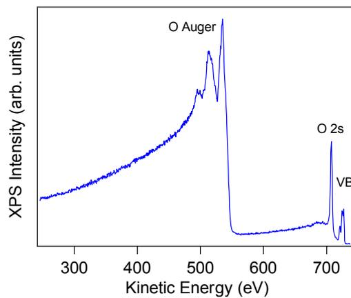
**Figure S2.** XPS survey of 2 wt% FeOOH nanoparticles dispersed in water taken with a photon energy of 708 eV. No detectable carbon signature expected at about 415 – 425 eV kinetic energy range is present indicating that the nanoparticles are ligand free as declared by the producing company (PlasmaChem).
