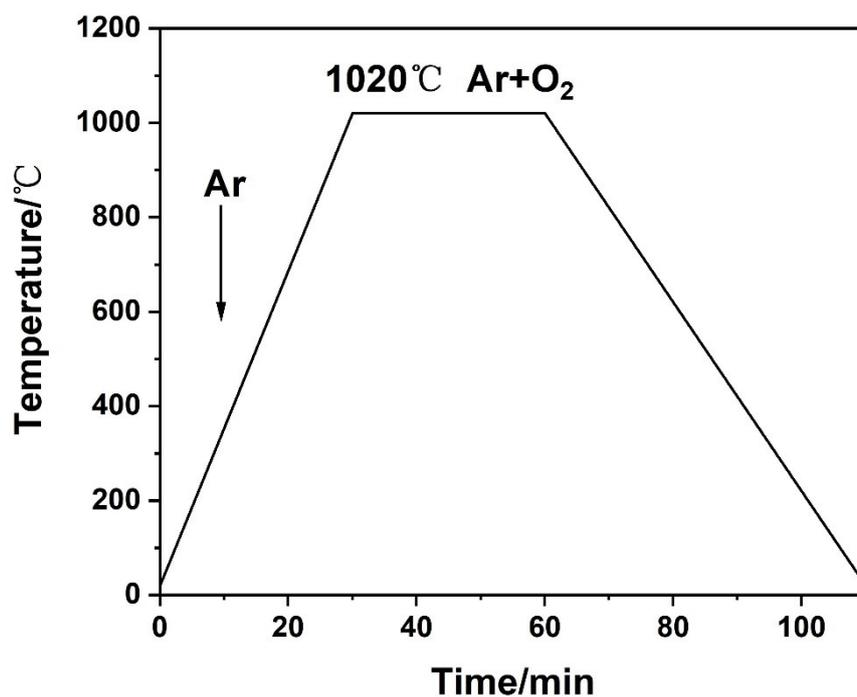
**Figure S2.** Schematic diagram of heating process of CVD system
