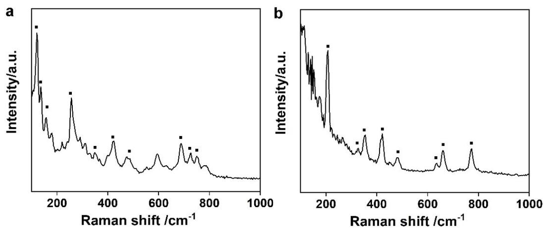
**Figure S5.** Raman spectrum of α-Ga<sub>2</sub>O<sub>3</sub> and β-Ga<sub>2</sub>O<sub>3</sub>, respectively.
