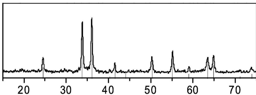
Figure S7. XRD spectrum of  $\alpha$ -Ga<sub>2</sub>O<sub>3</sub> crystals.
