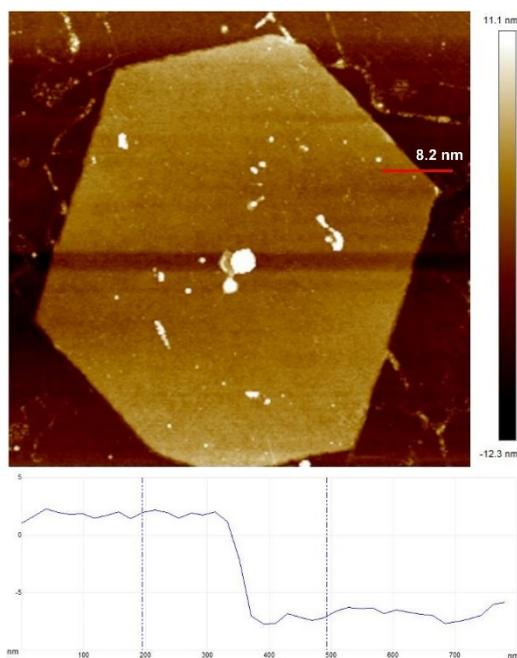
**Figure S4.** Thickness measurement of Ga<sub>2</sub>O<sub>3</sub> sheet. It is noted that the thickness is around 8 nm.
