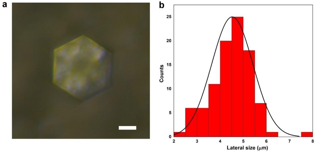
**Figure S3.** (a) Optical images of  $\alpha$ - $\text{Ga}_2\text{O}_3$  crystals. (b) Statistical distributions of the lateral size 2D ultrathin  $\text{Ga}_2\text{O}_3$  crystals. The scale bar in (a) is 2  $\mu\text{m}$ .
