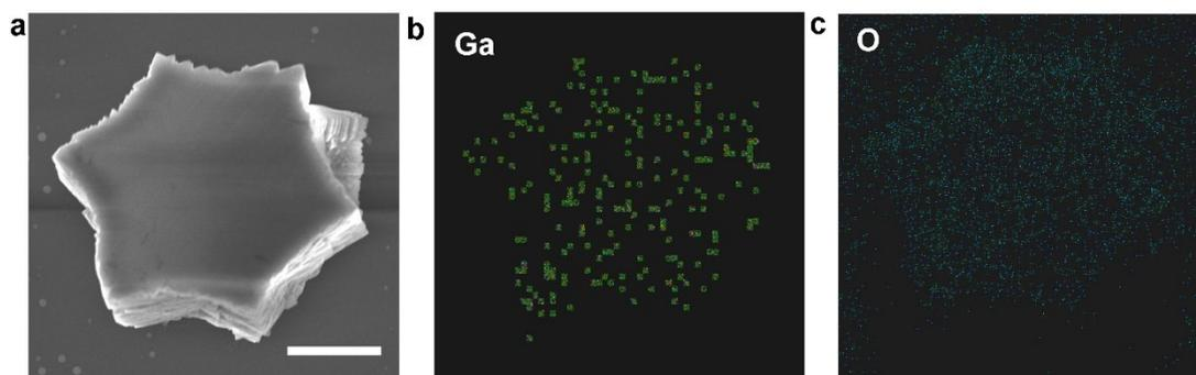
**Figure S6.** EDS mapping of the as grown Ga<sub>2</sub>O<sub>3</sub> crystal. (a) SEM images of the hexagonal  $\alpha$ -Ga<sub>2</sub>O<sub>3</sub> crystal.(b), (c) EDS elemental mapping of Ga and O. The scale bar is 2  $\mu$ m.
