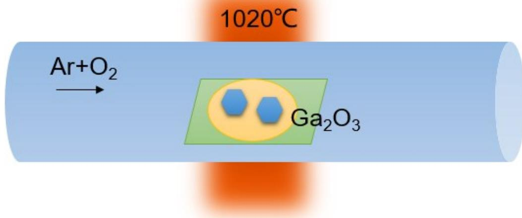
**Figure S1.** Sketch map of the CVD procedure for 2D ultrathin  $\text{Ga}_2\text{O}_3$  crystals at the ambient pressure.
