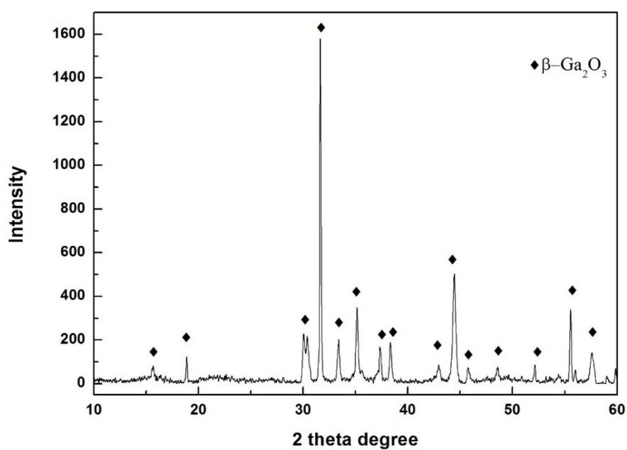
**Figure S9.** XRD spectrum of  $\beta$ - $\text{Ga}_2\text{O}_3$  crystals.
