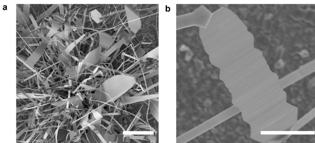
**Figure S8.** (a), (b) SEM images of  $\beta$ - $\text{Ga}_2\text{O}_3$  nanosheets. The scale bars in (a) is 20  $\mu\text{m}$  and in (b) is 5  $\mu\text{m}$ .
