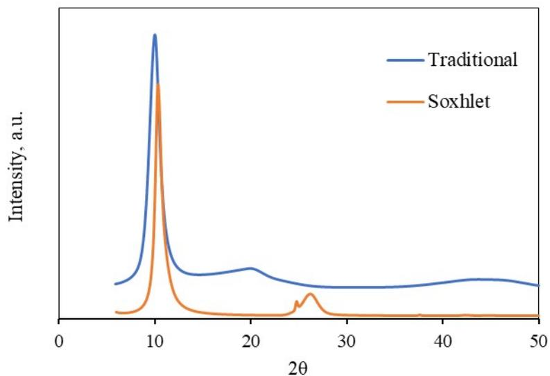
**Figure S3:** X-ray Diffraction (XRD) spectra of Soxhlet- and traditionally washed graphite-oxide. The  $10^\circ$  and  $20/26^\circ$   $2\theta$  correspond to the (002) inter-layer plane of GO and graphite, respectively.
