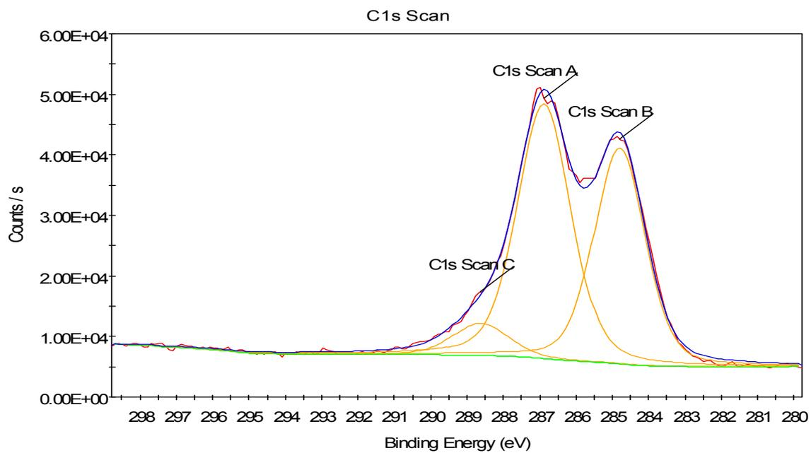
**Figure S5:** C1s scan and fitting for the Soxhlet washed GO.
