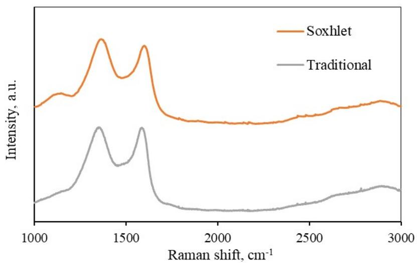
**Figure S2:** Raman spectra of Soxhlet- and traditionally- washed GO stimulated with 532 nm wavelength beam.
