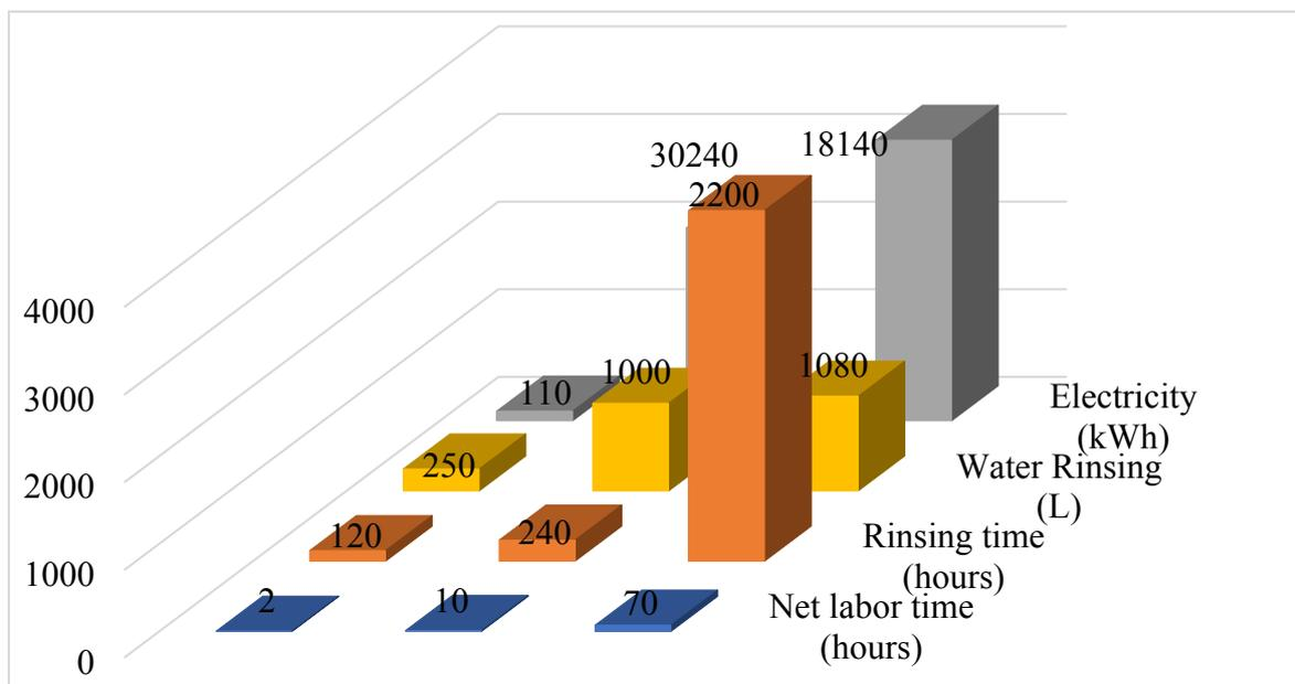
**Figure S7.** Comparison of rinsing requirements at different methods for 1kg graphite-oxide.
