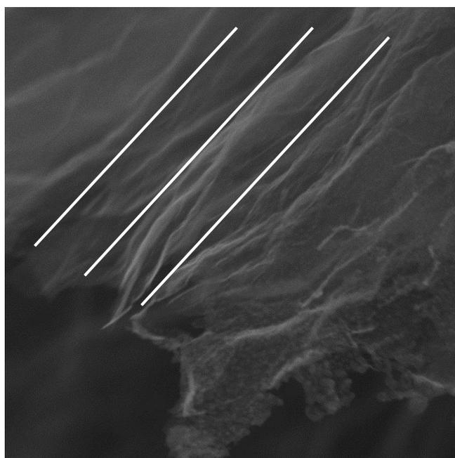
**Figure S6:** SEM image showing layered structure of reduced Graphite-oxide.
