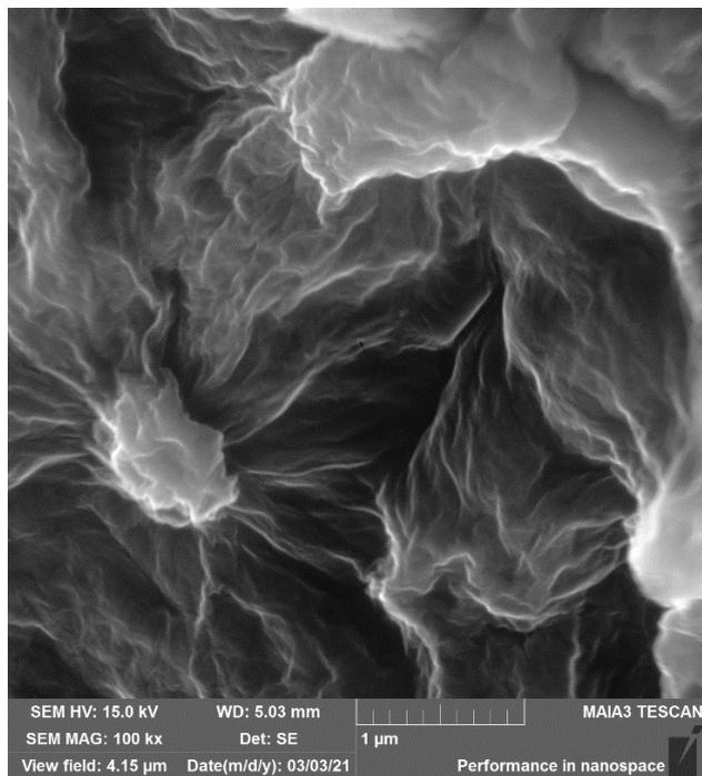
**Figure S1:** Typical scanning electron microscope (SEM) image of graphite-oxide after washing with Soxhlet extractor.
