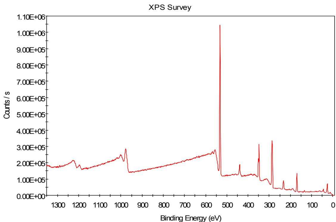
**Figure S4:** XPS survey for elemental analysis of the Soxhlet washed GO
