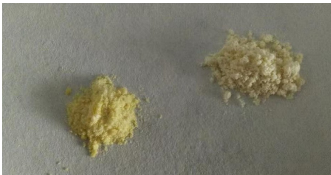
Fig. S13 The graph of Compound 1 died under the air condition (left) and vacuum condition (right).
