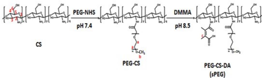
**Figure S8.** Synthesis of PEG-CS-DA.
