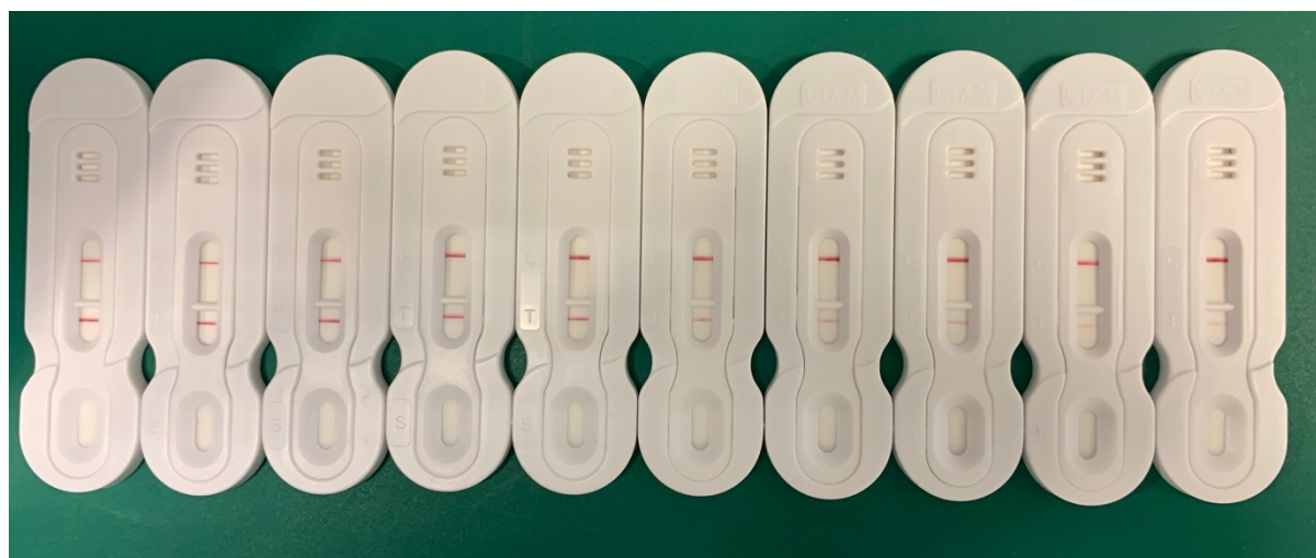
Fig S9: Results of CTX-M in vitro screen: Concentration range of 1.2 \mu M (left) – 1.2 fM (right), incremental serial dilutions of 10-fold.
