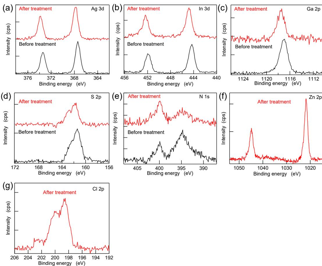
**Fig. S7** XPS spectra of the AIGS/Ga<sub>y</sub>S core/shell-like QDs before (black curves) and after (red curves) the ZnCl<sub>2</sub> treatment: (a) Ag 3d, (b) In 3d, (c) Ga 2p, (d) S 2p, (e) N 1s, (f) Zn 2p, and (g) Cl 2p.
