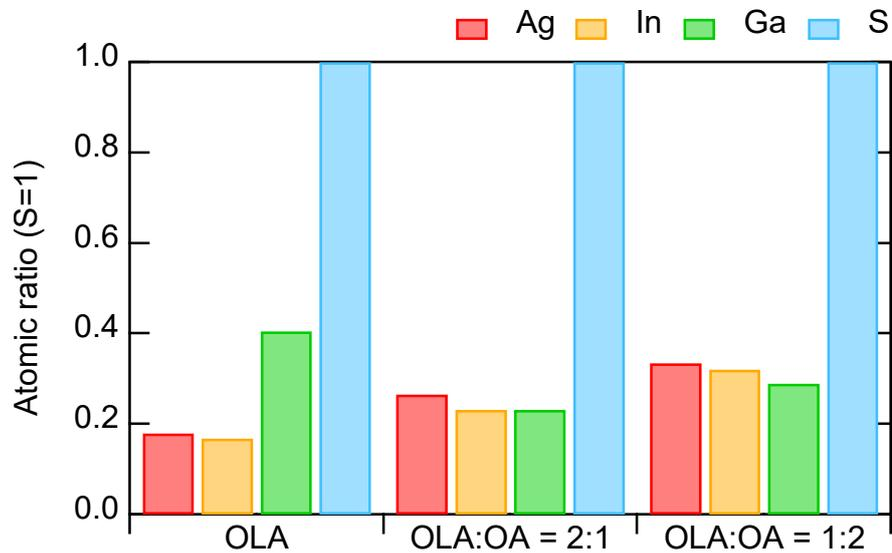
**Fig. S3** Atomic ratios (sulfur basis) obtained via the EDX–SEM analysis for the AIGS QDs synthesized with various surface ligands.
