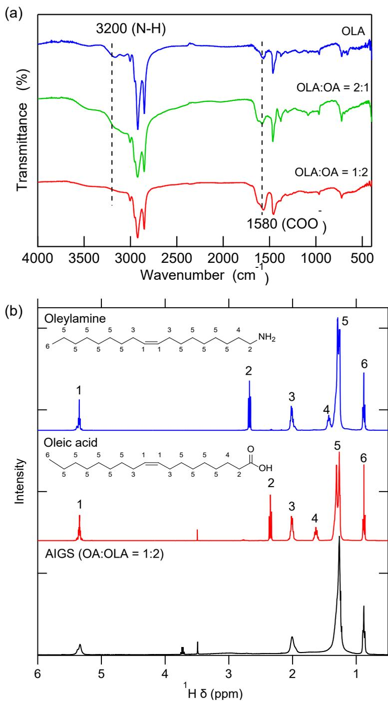
**Fig. S2** (a) FT-IR spectra of the AIGS QDs synthesized with OLA only and an OLA:OA mixture (with ratios 2:1 and 1:2). (b) <sup>1</sup>H NMR spectra (chloroform-d) of free OLA and OA as well as of AIGS QDs synthesized in an OLA:OA mixture solvent (2:1).
