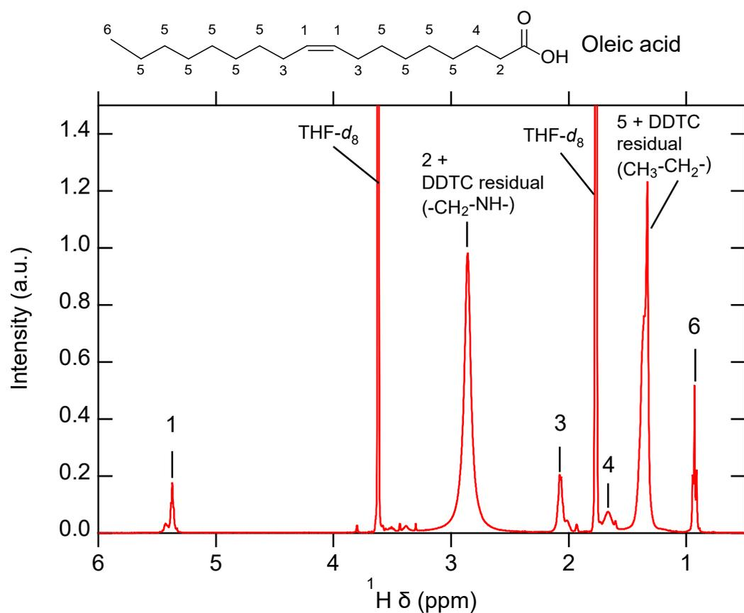
**Fig. S4** (a)  $^1\text{H}$  NMR spectra ( $\text{THF-}d_8$ ) of the white precipitate that was generated after the  $\text{ZnCl}_2$  treatment of the AIGS QDs synthesized in the OLA:OA mixture solvent (with ratio 2:1).
