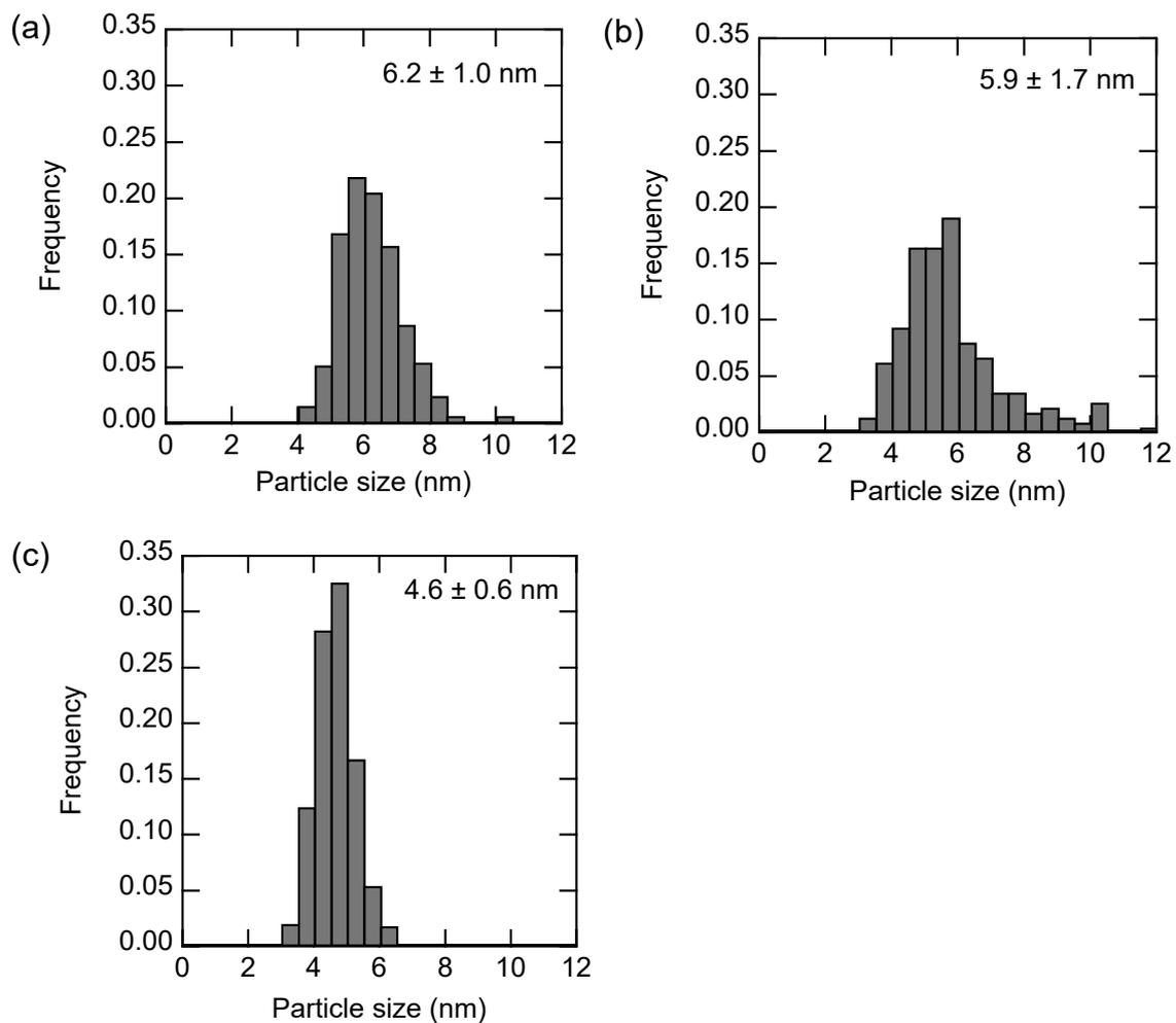
**Fig. S1** Corresponding size distributions of Fig. 1(a–c) for the as-synthesized AIGS QDs in different solvents: (a) OLA, (b) OLA:OA = 2:1, and (c) OLA:OA = 1:2.
