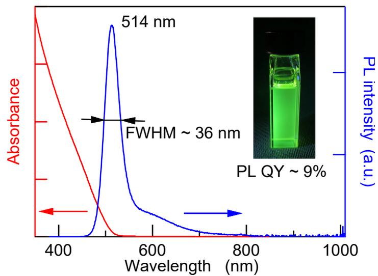
**Fig. S6** UV-vis absorption and PL spectra of the AIGS/Ga<sub>y</sub>S core/shell-like QDs with the inset photograph showing the QD solution under UV radiation (365 nm); the photographed QD solution has a PL QY of approximately 9%, as labeled in the figure.
