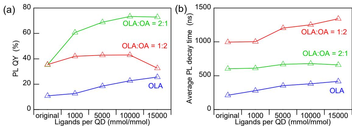
**Fig. S5** Change in (a) the PL QY values and (b) the average PL decay times of the AIGS QDs synthesized using various ligands (OLA, OLA:OA = 2:1, and OLA:OA = 1:2) before and after the  $\text{ZnCl}_2$  treatment at 1,000–15,000 ligands/QD.
