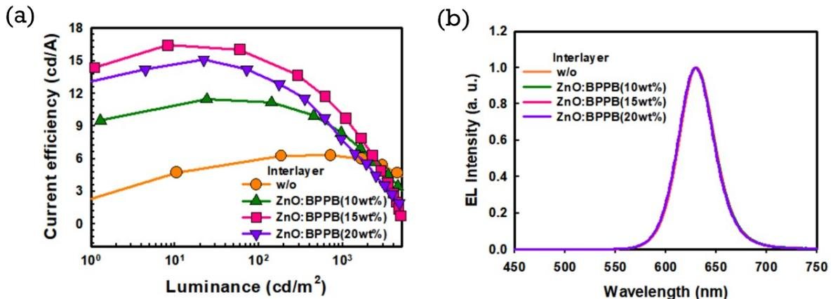
**Fig. S7** (a) Current efficiency versus luminance characteristics (b) Electroluminescent (EL) spectrum of InP-QLED devices without (w/o) and with interlayers.
