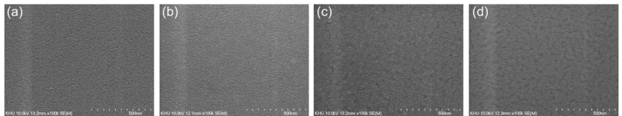
**Fig. S5** SEM images of the samples (a) ZnO (b)ZnO/ZnO:BPPB(10wt%) (c) ZnO/ZnO:BPPB(15wt%), and (d)ZnO/ZnO:BPPB(20wt%).
