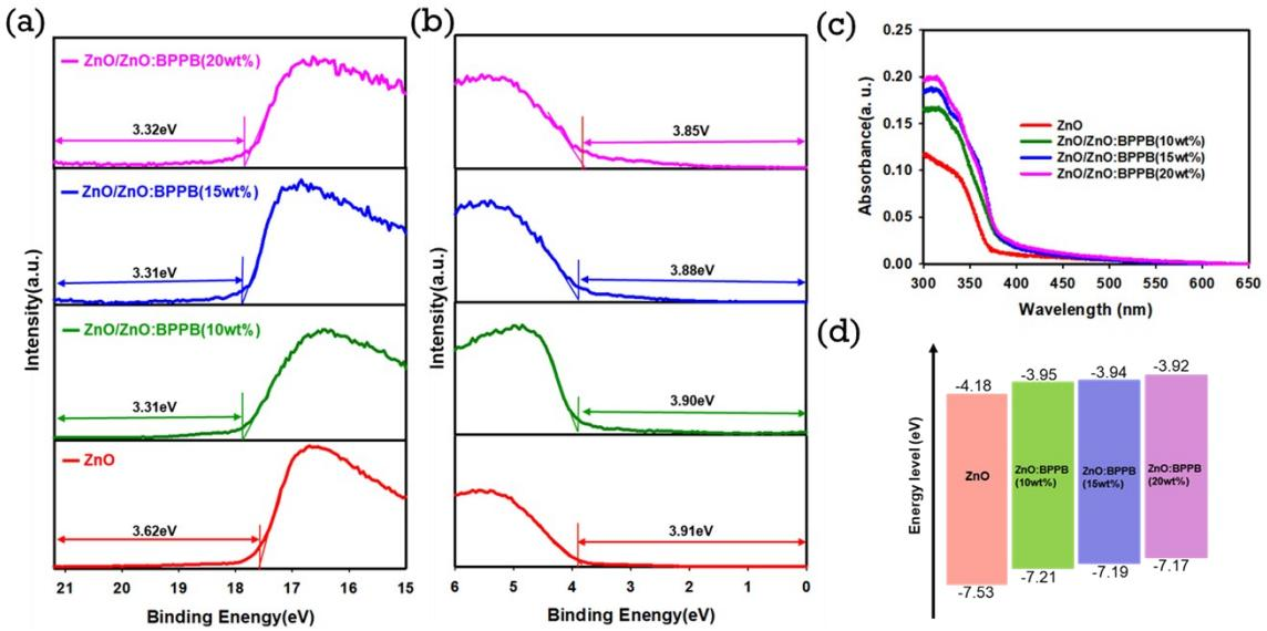
**Fig. S6** UPS spectra of the samples ZnO, ZnO/ZnO:BPPB(10wt%) ZnO/ZnO:BPPB(15wt%) and ZnO/ZnO:BPPB(20wt%) (a) Secondary electron cutoff regions (b) valance band edge regions (c) UV-Vis absorption spectra (d) Energy band diagram.
