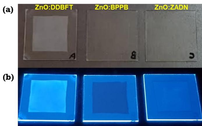
**Fig. S2** Photographs of the different small molecule ETLs blended in ZnO (ZnO:DDBFT, ZnO:BPPB, ZnO:ZADN) (a) under normal light (b) under UV light.
