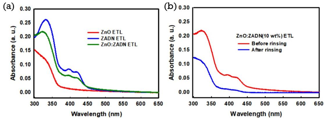
**Fig. S3** (a) UV-Vis absorption spectra of ZnO, ZADN and ZnO:ZADN(10wt%) films. (b) UV-Vis absorption spectra of ZnO:ZADN(10wt%) ETL film before and after octane rinsing.
