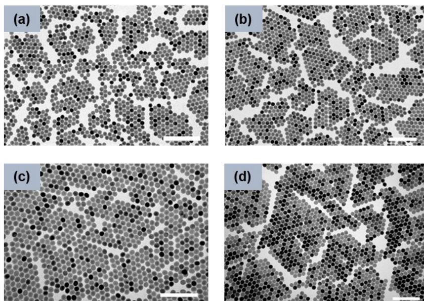
**Figure S1. TEM images of core samples.** (a)  $\text{NaYF}_4:20\%\text{Yb}^{3+}$ , 2%  $\text{Er}^{3+}$  core nanoparticles. (b)  $\text{NaYF}_4:30\%\text{Yb}^{3+}$ , 8%  $\text{Er}^{3+}$  core nanoparticles. (c)  $\text{NaYF}_4:30\%\text{Yb}^{3+}$ , 2%  $\text{Er}^{3+}$  core nanoparticles. (d)  $\text{NaYF}_4:20\%\text{Yb}^{3+}$ , 1.5%  $\text{Er}^{3+}$  core nanoparticles. Scale bar: 200 nm.
