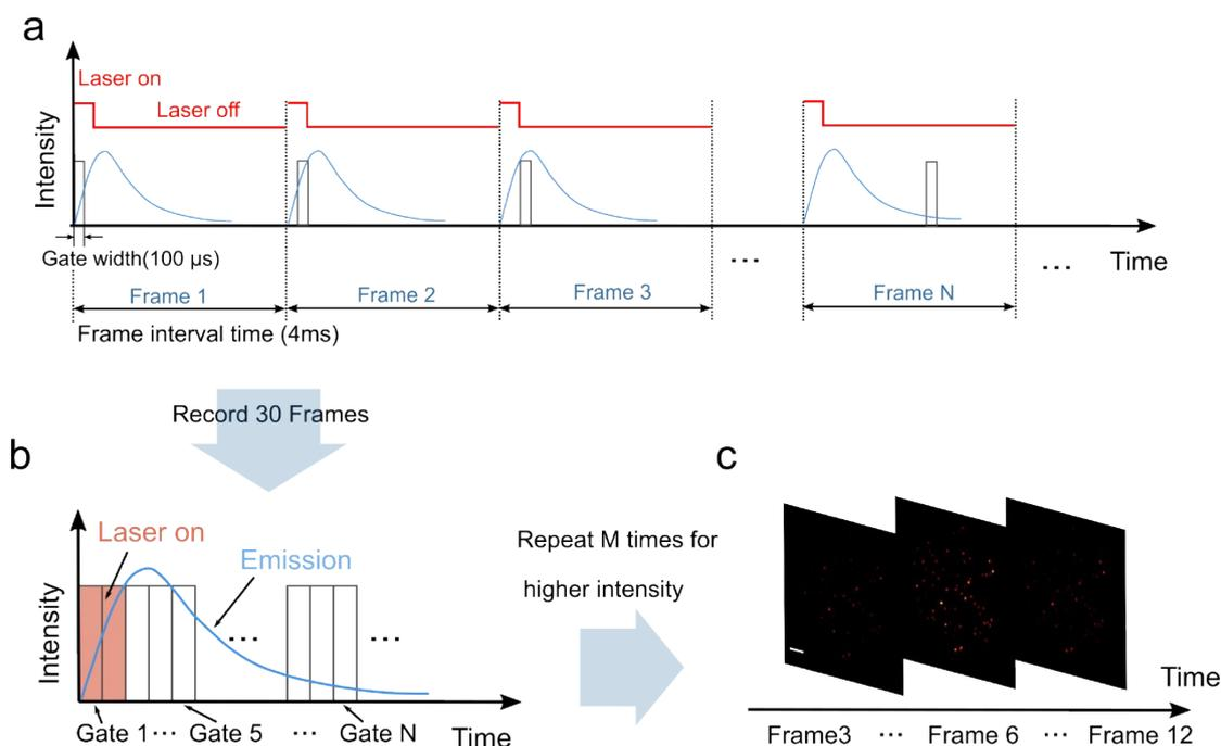
**Figure S5.** The principle for time-gated wide-field imaging. (a) The camera is gated with an exposure time of 100  $\mu$ s, and in each frame, only a gated image can be detected. The imaging gate will be shifted to the next 100  $\mu$ s. The lifetime curve/images (b) can be reconstructed by 30 frames. To obtain a better signal-to-noise ratio, we repeat the process for M times (e.g M=7500 for TR-SIM, and M=3000 for TR-WF) and integrate the signal to obtain a series of time-resolved images (c).
