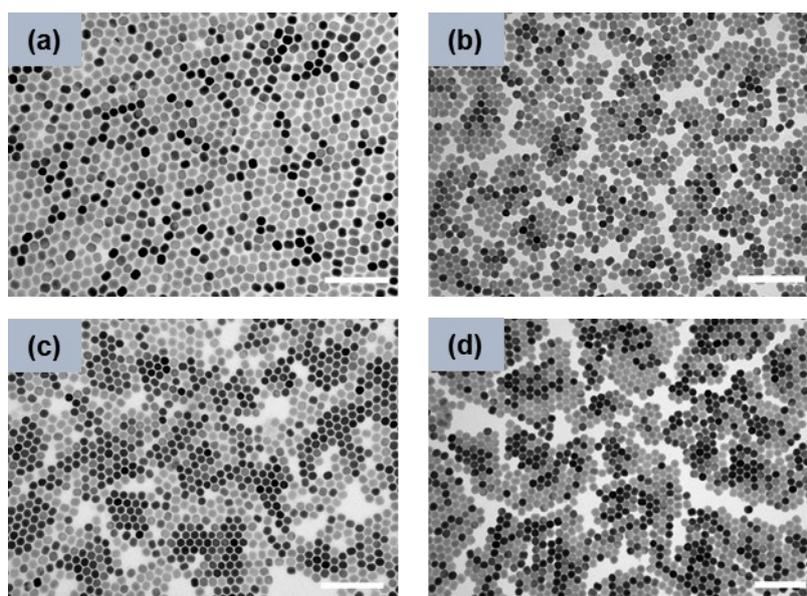
**Figure S2. TEM images of core-shell nanoparticles.** (a)  $\text{NaYF}_4:20\%\text{Yb}^{3+}$ , 2%  $\text{Er}^{3+}$  @  $\text{NaYF}_4:5\%\text{Yb}^{3+}$  nanoparticles. (b)  $\text{NaYF}_4:30\%\text{Yb}^{3+}$ , 8%  $\text{Er}^{3+}$  @  $\text{NaYF}_4:5\%\text{Yb}^{3+}$
