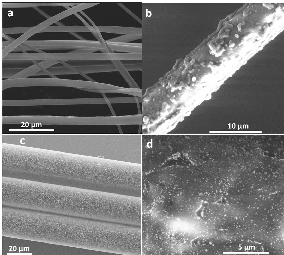
**Fig. S1** (a) SEM image the jetted PLGA fibers prior to seed particle deposition. (b) a PLGA fiber after seed particle deposition and silver enhancement to enable easy SEM imaging. (c) SEM image of Nylon fibers coated with seed particles after silver enhancement. (d) SEM image of a higher magnification showing a small region of a Nylon fiber surface with the silver enhanced seed particles, demonstrating the uniform distribution of seeds.
