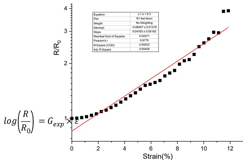
**Fig. S4** Resistance vs. strain curve for the first stretch cycle of the sample presented in Fig. 4b. The fit to a linear curve in a log-scale representation indicates a nearly exponential dependence with a slope of  $G_{exp} \sim 4.8$ , representing the exponential Gauge Factor. A similar exponential dependence can be observed also in Fig. S3, for the initial part of the stretch (up to  $\sim 20\%$  elongation).
