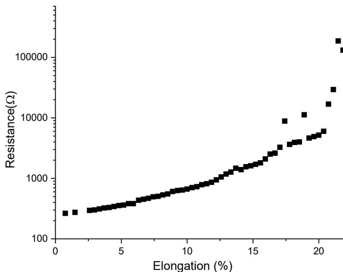
**Fig. S3** Resistance vs. strain stretching curve of a nylon fibre coated with the metal NW network. This was the sample that achieved the highest strain while still electrically conducting.
