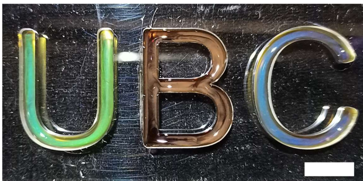
Fig. S18 GO photonic suspensions in pure poly(APMS-co-DMS) copolymer liquids were injected into a plastic mold to make an “UBC” pattern with different reflection colors. Scale bar: 1 cm.
