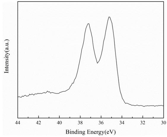
Fig.S7 XPS spectrum for W of the composite after the photocatalytic degradation
