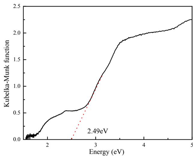
Fig S9 K-M function against energy E of SiW<sub>12</sub> polyoxometalate
