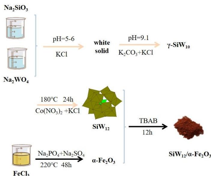
Scheme S1: the preparation process of  $\text{SiW}_{12}/\alpha\text{-Fe}_2\text{O}_3$  nanocomposite
