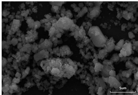
Fig. S8 The IR spectra and SEM image of the SiW<sub>12</sub>/3%α-Fe<sub>2</sub>O<sub>3</sub> composite after photocatalytic degradation
