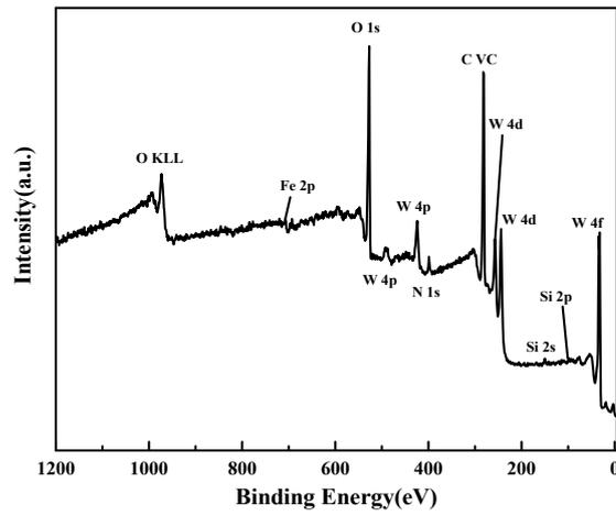
Fig.S2 The full survey spectrum of the  $\text{SiW}_{12}/\alpha\text{-Fe}_2\text{O}_3$  composite
