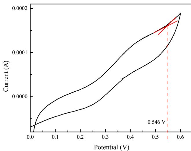
Fig S10 The cyclic voltammograms of SiW<sub>12</sub> polyoxometalate
