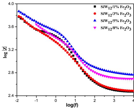
Fig.S3 The Bode plots of composites with different amount of  $\text{Fe}_2\text{O}_3$
