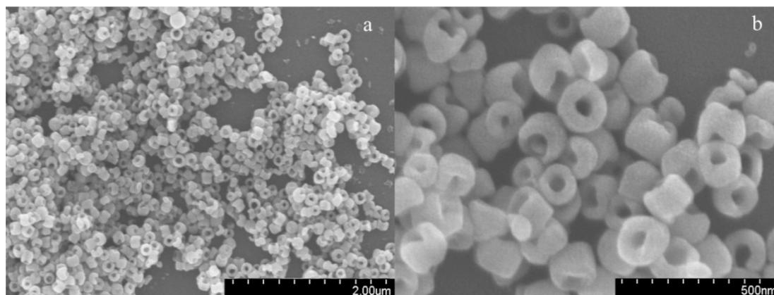
Fig.S1 SEM images of  $\alpha$ -Fe<sub>2</sub>O<sub>3</sub> nanoring
