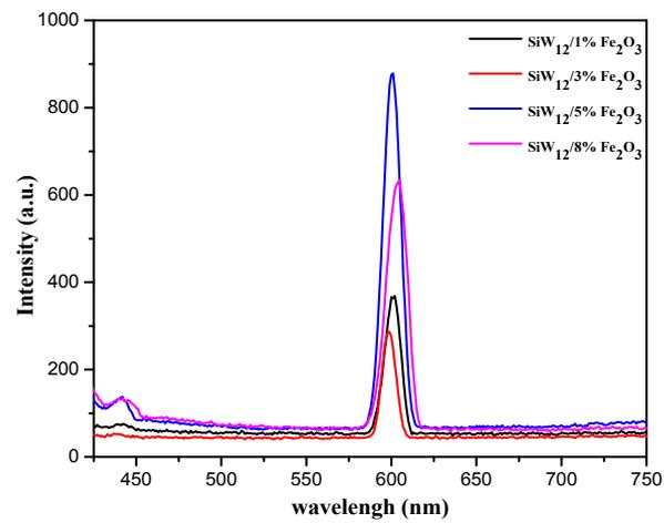
Fig.S4 The PL spectra of composites with different amount of  $\text{Fe}_2\text{O}_3$
