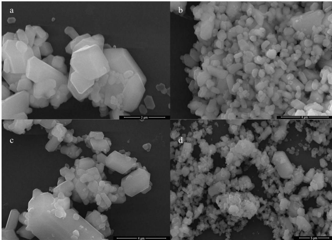
Fig.S5 SEM images of  $\text{SiW}_{12}/\alpha\text{-Fe}_2\text{O}_3$  with different ratio (a)  $\text{SiW}_{12}/1\%\alpha\text{-Fe}_2\text{O}_3$ , TBAB 10ml. (b)  $\text{SiW}_{12}/3\%\alpha\text{-Fe}_2\text{O}_3$ , TBAB 10ml. (c)  $\text{SiW}_{12}/5\%\alpha\text{-Fe}_2\text{O}_3$ , TBAB 10ml. (d)  $\text{SiW}_{12}/8\%\alpha\text{-Fe}_2\text{O}_3$ , TBAB 10ml
