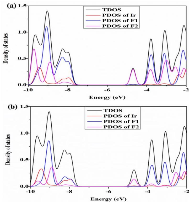
Fig S4 Partial and total density of states (PDOS and TDOS) obtained at B3LYP/6-31G\*/SDD level for studied complexes **IRC-1** and **IRC-2**.
