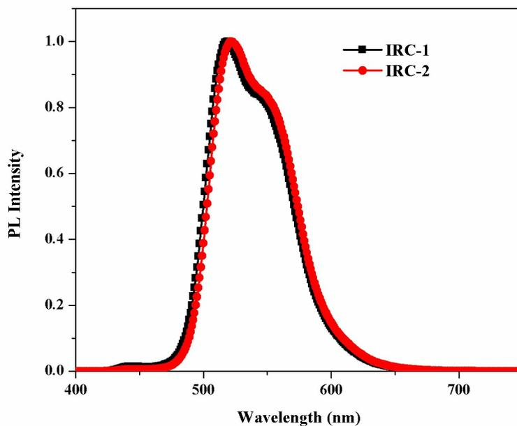
**Fig S1** Electronic emission spectra of **IRC-1** and **IRC-2** in CH<sub>2</sub>Cl<sub>2</sub> solution.
