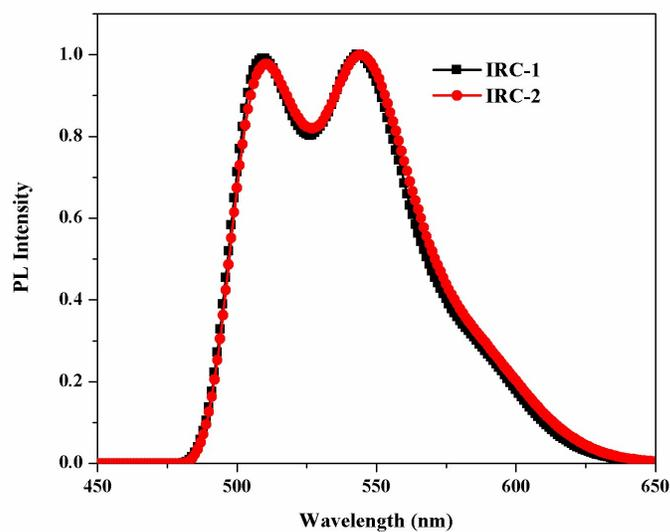
Fig S3 PL spectra of **IRC-1** and **IRC-2** at low temperature 77 K
