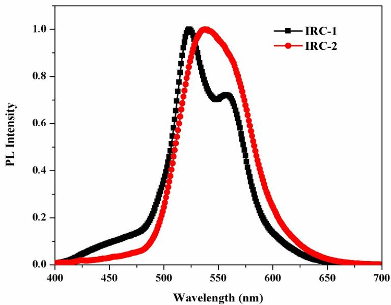
**Fig S2** Emission spectra of **IRC-1** and **IRC-2** in neat thin films at room temperature.
