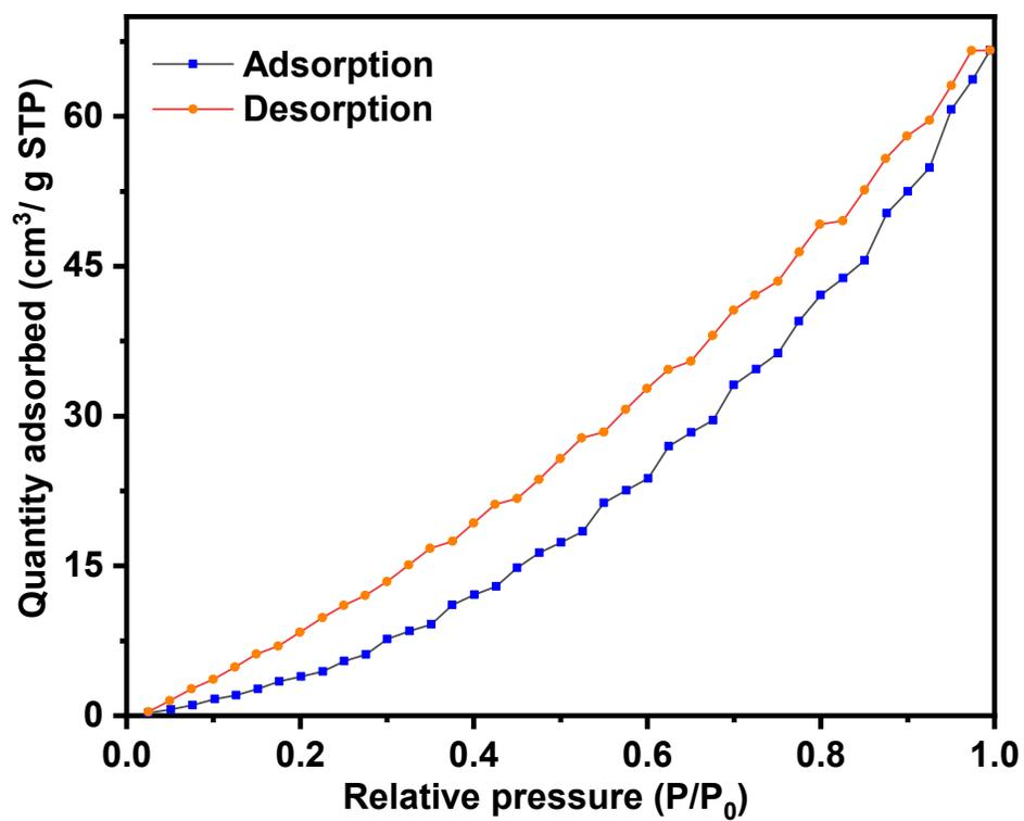
Fig. S5: N<sub>2</sub> sorption plot of compound 1.
