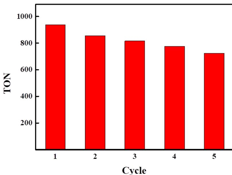
Fig. S1. Recyclability of PdAg/TEDA-MIL-101-NH<sub>2</sub> catalyst during the hydrogenation of CO<sub>2</sub> into formic acid. Reaction condition: 20 mg catalyst, the total pressure of 5.0 MPa (CO<sub>2</sub> : H<sub>2</sub> = 1 : 1, volume ratio) at 70 °C for 10 h.
