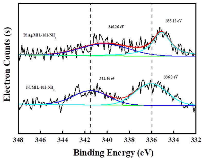
Fig. S5. The Pd 3d XPS of Pd/MIL-101-NH<sub>2</sub> and PdAg/MIL-101-NH<sub>2</sub>.
