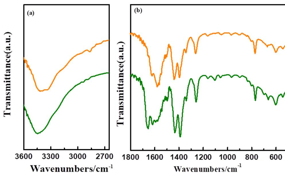
Fig. S4. Partial enlarged view of fresh and recycled catalysts FT-IR spectra. (a) High wavenumbers; (b) Low wavenumbers of fresh PdAg/TEDA-MIL-101-NH<sub>2</sub> (green); recycled PdAg/TEDA-MIL-101-NH<sub>2</sub> (yellow)
