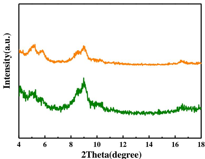
Fig. S2. The PXRD pattern of PdAg/TEDA-MIL-101-NH<sub>2</sub> fresh (green) and recycled (yellow) catalysts.
