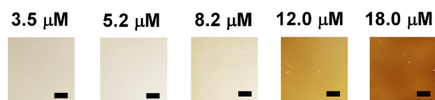
Figure S7. Photographs of the quercetin/DETA-coated Ti/TiO 2 substrates. The quercetin concentration was varied, and the scale bars represent 2 mm.
