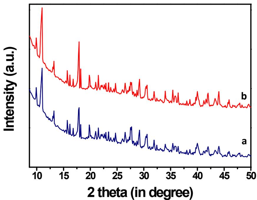
Figure S4: PXRD of reused catalyst (a) and activated catalyst (b).
