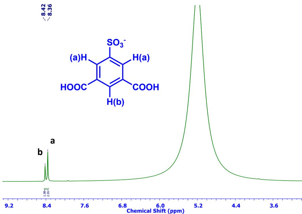
Figure S6:  $^1\text{H}$  NMR of La-5-SIP-MOF after acid digestion.
