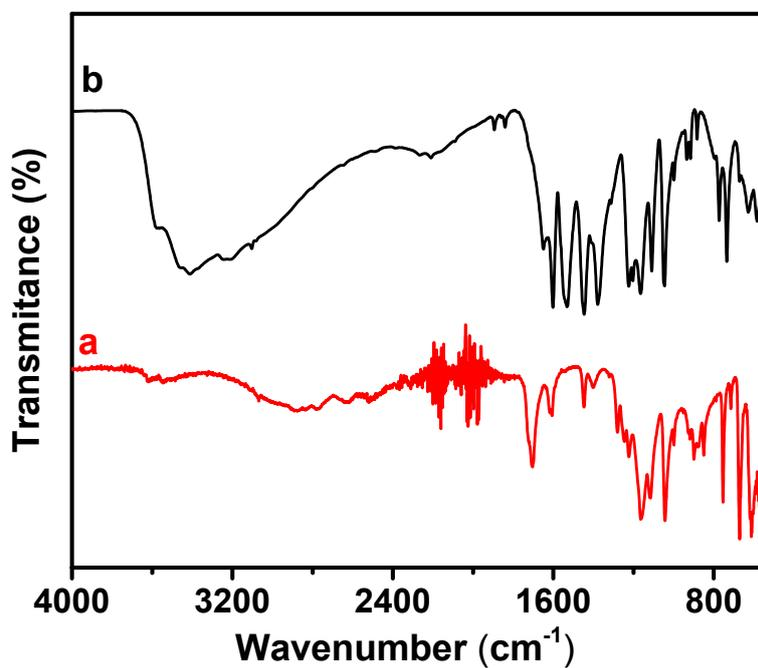
Figure S2: FT-IR spectra of 5-NaSIP ligand (a) and La-5-SIP-MOF (b).
