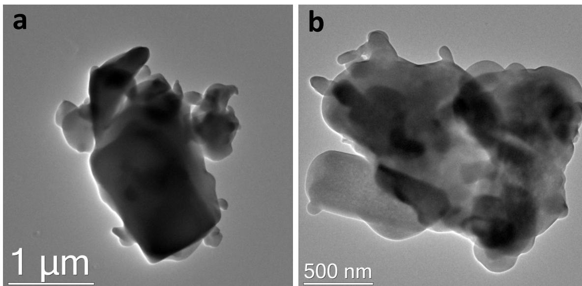
**Figure S7:** UHR-TEM images of La-5-SIP-MOF: a. before catalysis; b. after catalysis.
