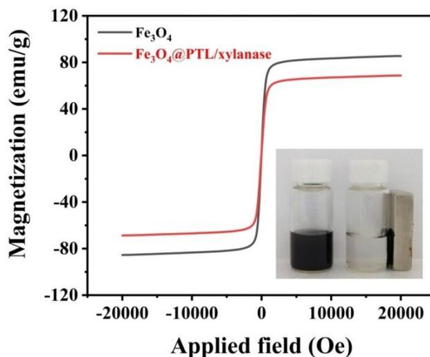
**Figure S1.** The magnetic hysteresis loops of  $\text{Fe}_3\text{O}_4$  NPs (black line) and  $\text{Fe}_3\text{O}_4@PTL/xylanase$  nanocomposites (red line), and the inset shows the pictures of nanocomposite solution before and after magnetic separation.
