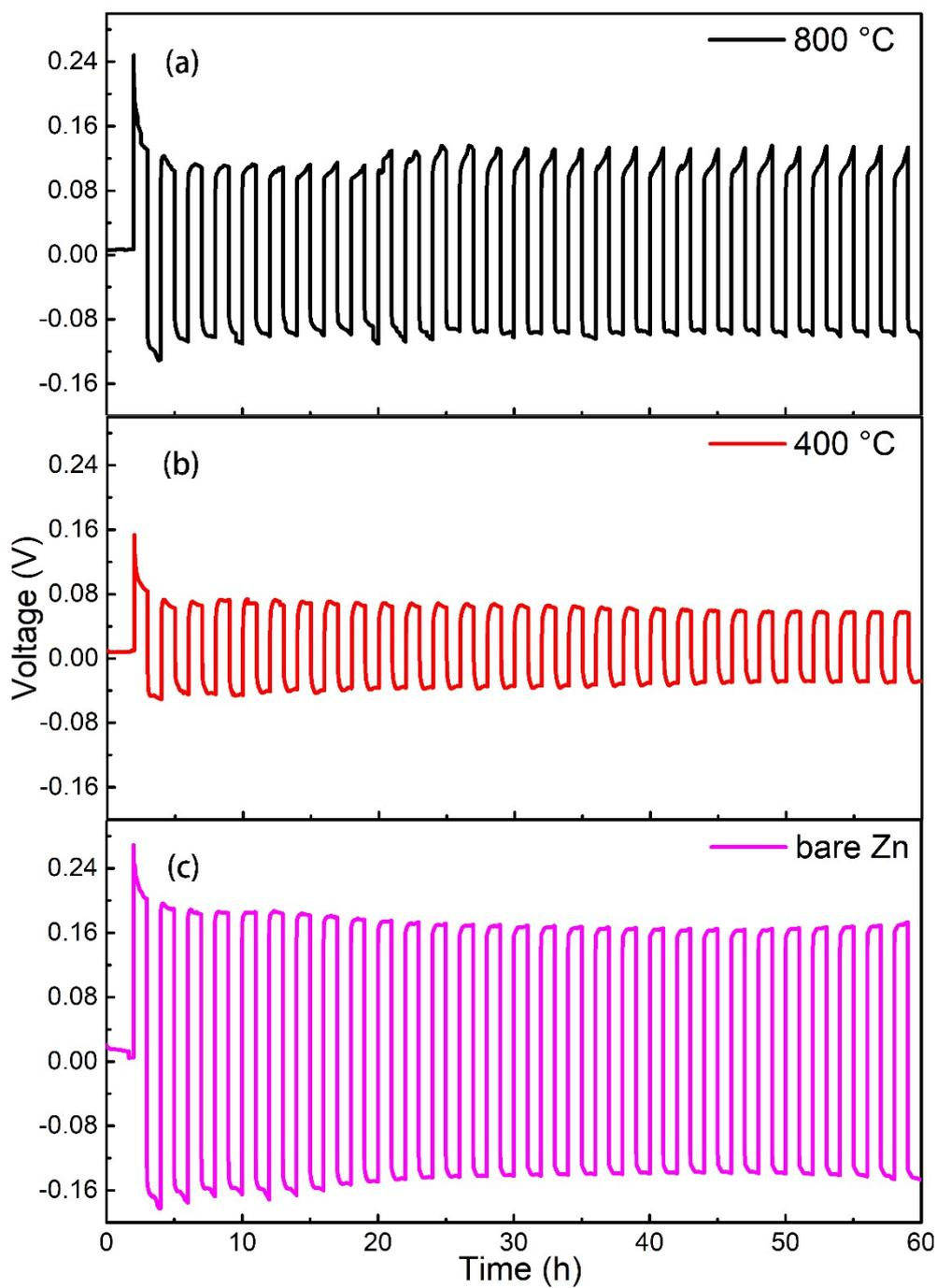
**Figure S6** Galvanostatic cycling performances of Zn/ZnSO<sub>4</sub>/Zn symmetric cells contained fabricated cocoon with the sintered temperature of (a) 800 °C, (b) 400°C and (d) bare Zn at a current density of 0.25 mA cm<sup>-2</sup> after 30 cycles.
