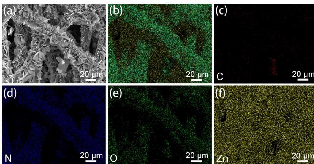
**Figure S5** The elemental mapping of the cocoons at the temperature of 800 °C after cycling in ZBs-800.
