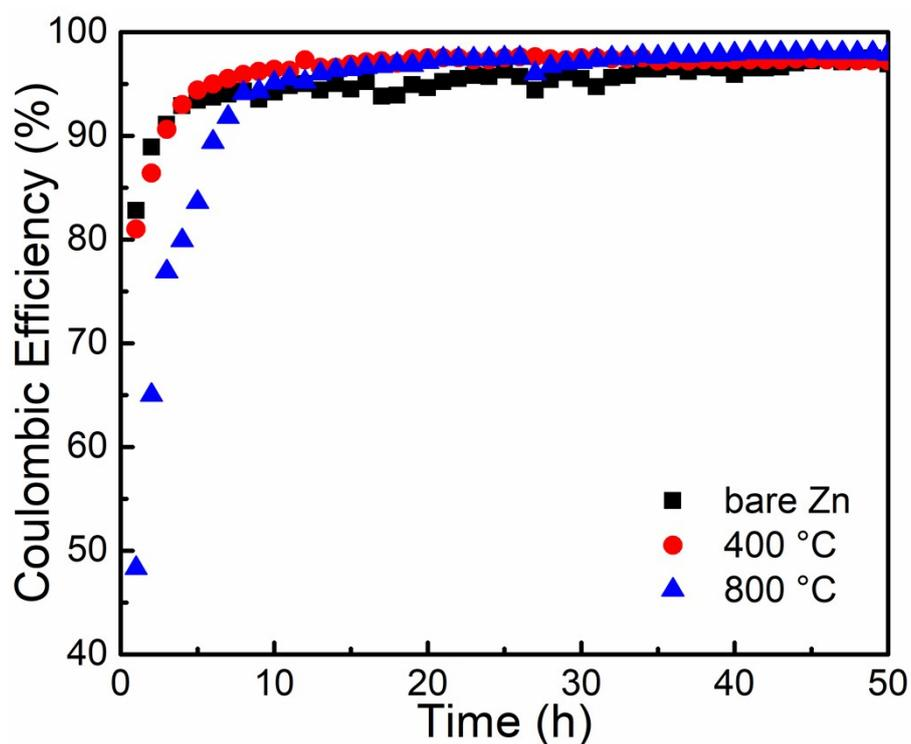
**Figure S8** Coulombic efficiencies of Zn|Cu batteries without cocoon and with cocoons under different heating process at a current density of 0.25 mA cm<sup>-2</sup>.
