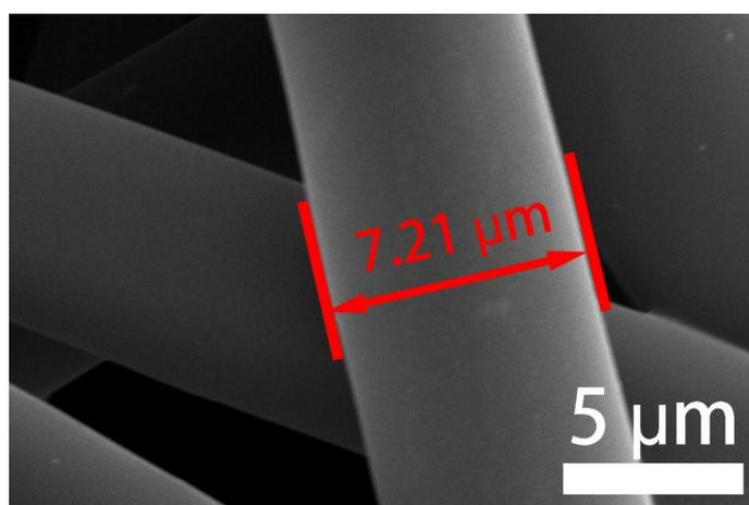
**Figure S2** The SEM image of silk cocoons carbonized under the heat treatment of  $800 \text{ }^{\circ}\text{C}$  (cocoon-800) and the diameter is about  $7.21 \text{ }\mu\text{m}$ .
