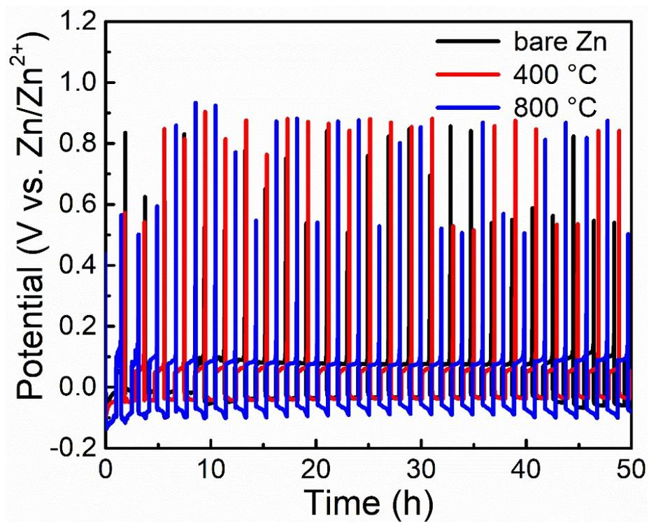
**Figure S9** Voltage profiles of charge/discharge process of Zn/Cu batteries without cocoon and with cocoons under different heating process at a current density of  $0.25 \text{ mA cm}^{-2}$ .
