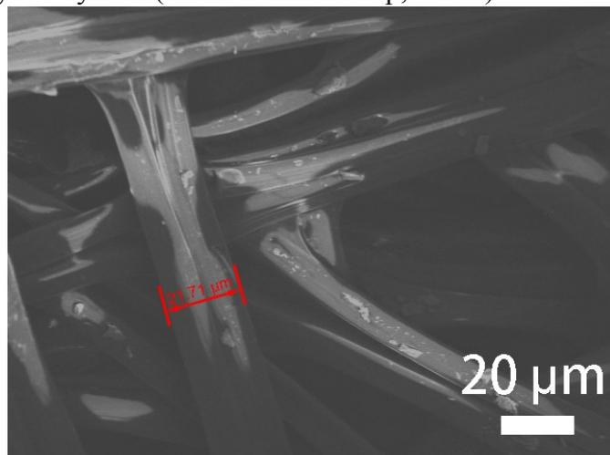
**Figure S1** The SEM image of original silk cocoons without heat treatment.
