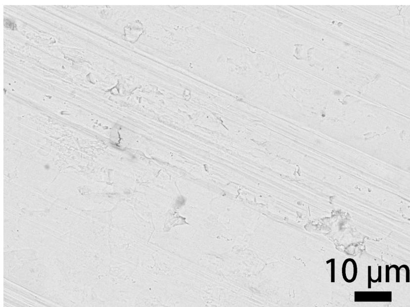
**Figure S4** The SEM image of the surface of Zn plate.
