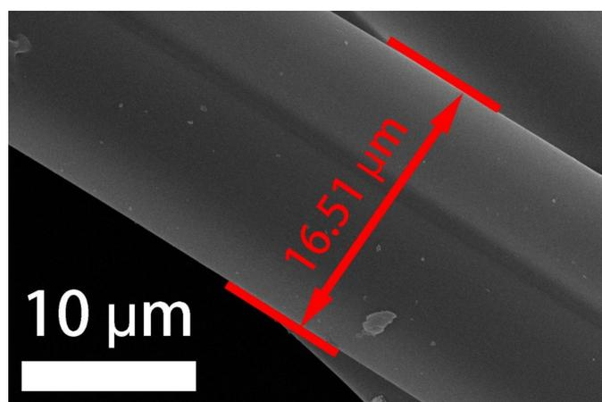
**Figure S3** The SEM image of silk cocoons carbonized under the heat treatment of  $400 \text{ }^{\circ}\text{C}$  (cocoon-400) and the diameter is about  $16.51 \text{ }\mu\text{m}$ .
