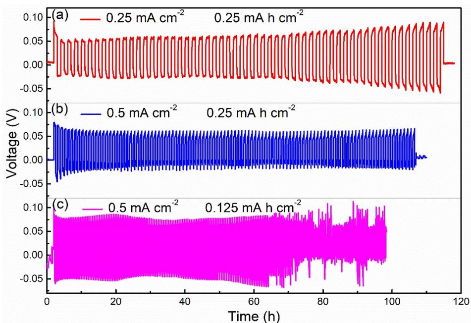
**Figure S7** Galvanostatic cycling performances of Zn|ZnSO<sub>4</sub>|Zn symmetric cells contained fabricated cocoons at 800 °C with different current density and capacity density: (a) 0.25 mA cm<sup>-2</sup>, 0.25 mA h cm<sup>-2</sup>, (b) 0.5 mA cm<sup>-2</sup>, 0.25 mA h cm<sup>-2</sup> and (c) 0.5 mA cm<sup>-2</sup>, 0.125 mA h cm<sup>-2</sup>.
