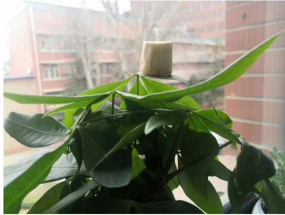
Fig. 4 A 10 cm 3 CSQS composite aerogel ( \rho = 0.16\text{mg/cm}^3 ) stands on the tip of leaf
