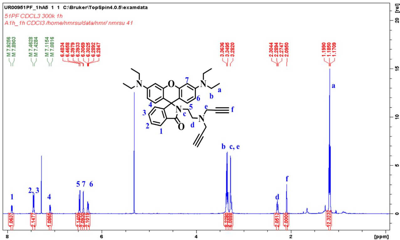
Figure S5. <sup>1</sup>H NMR spectra of compound 7 in CDCl<sub>3</sub>.
