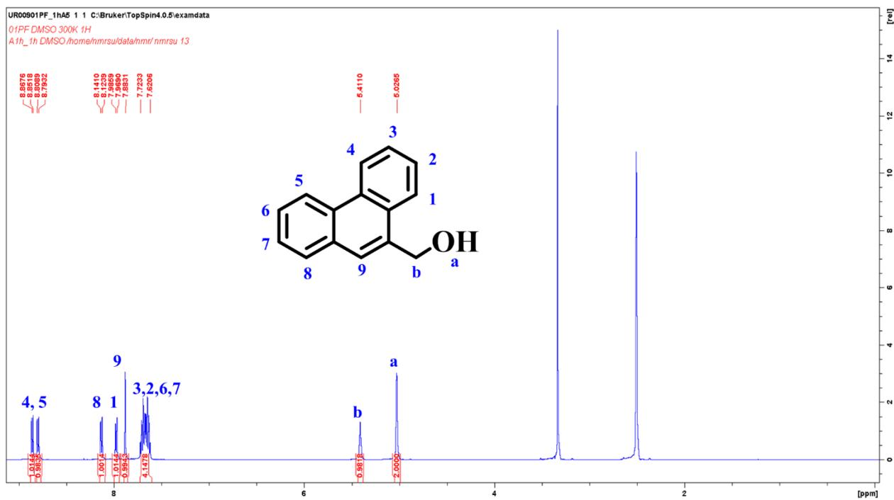
**Figure S1.**  $^1\text{H}$  NMR spectra of compound 2 in  $\text{DMSO-}d^6$ .
