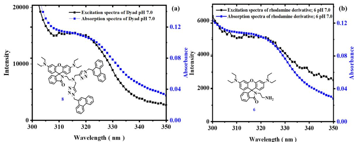
**Figure S16.** Overlay of the spectrally uncorrected fluorescence excitation spectra recorded at  $\lambda_{em} = 580$  nm and the corresponding absorption spectra at pH 7.0 (8.5  $\mu$ M) of (a) dyad **8** and (b) compound **6** in a THF- H<sub>2</sub>O mixture (1:1) in B-R buffer (25 mM). The reasonably good match between the absorption and excitation spectra underline the expected excitation wavelength independence of the fluorescence quantum yield of **8** and **6**.
