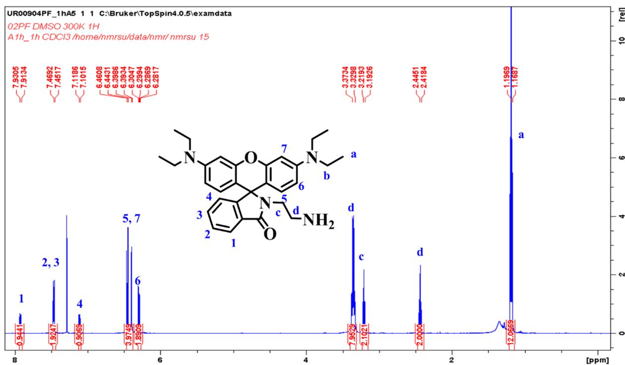
**Figure S4.**  $^1\text{H}$  NMR spectra of compound **6** in  $\text{CDCl}_3$ .
