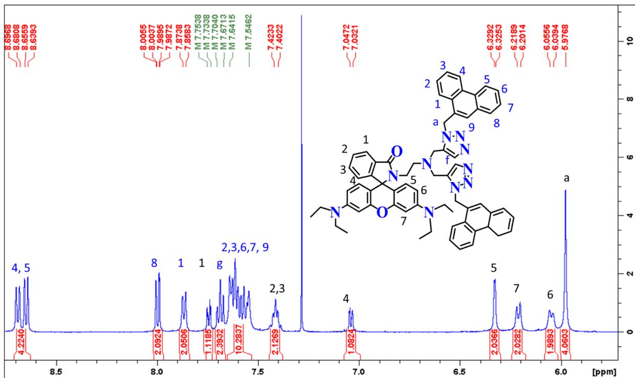
**Figure S7.** Magnified aromatic region of  $^1\text{H}$  NMR spectra of compound **8** in  $\text{CDCl}_3$ .
