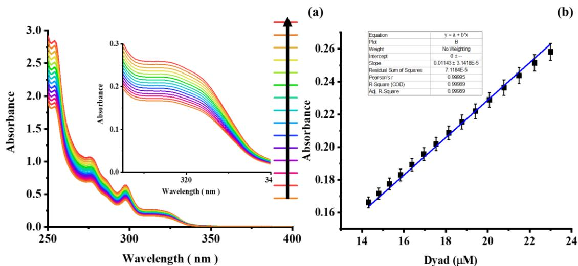
**Figure S13.** (a) Absorption spectra and (b) linear plot of the absorbance versus concentration of dyad **8** for calibration studies in a THF-H<sub>2</sub>O mixture (1:1) in a B-R buffer (25 mM).
