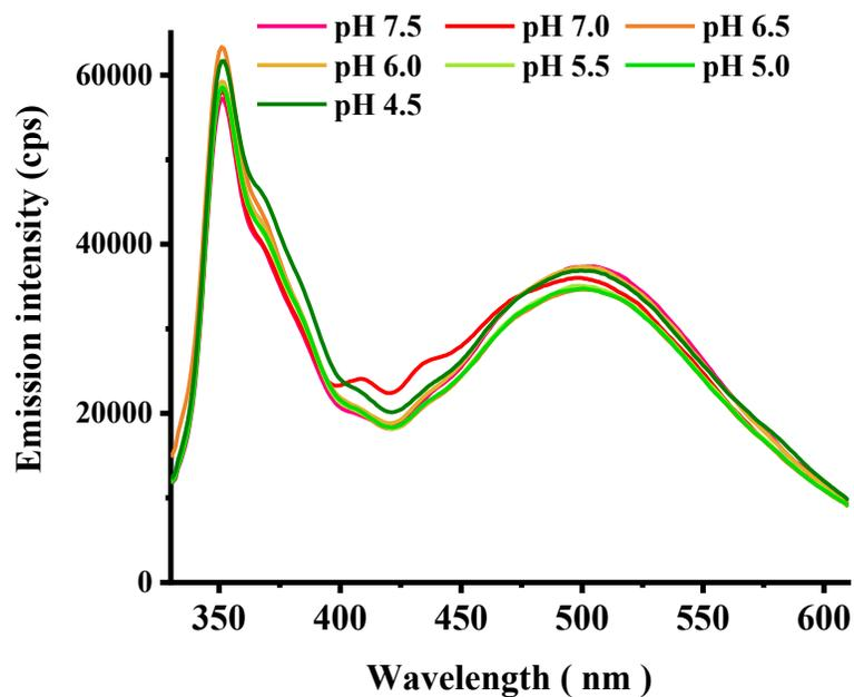
**Figure S14.** pH interaction studies of dyad; **8** (5 μM) at  $\lambda_{ex}$  315 in a THF-H<sub>2</sub>O mixture (1:1) in B-R buffer (25 mM).
