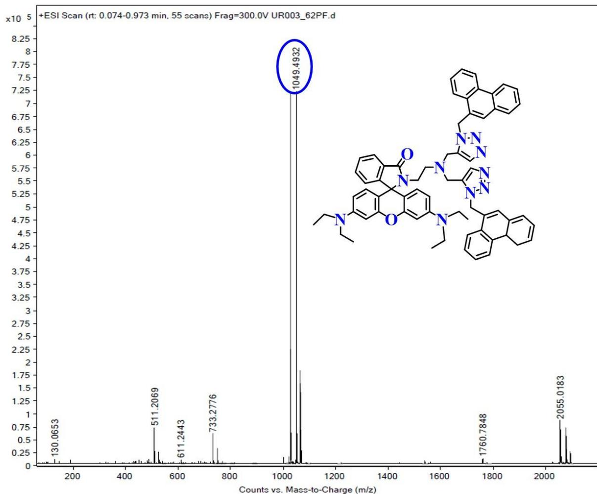
**Figure S9.** ESI-MS spectra of dyad **8** [ $8+\text{Na}^+$ ] in methanol.
