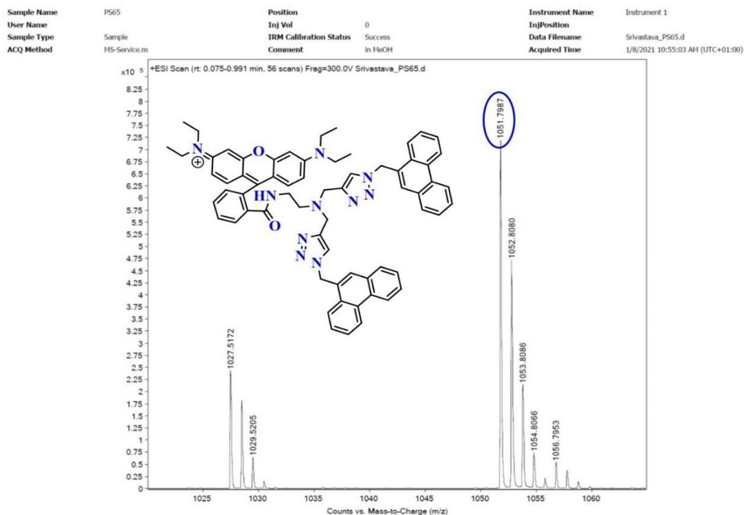
Figure S24. Magnified ESI-MS spectra of dyad  $[8 + Na^+ + H^+]$  in methanol.
