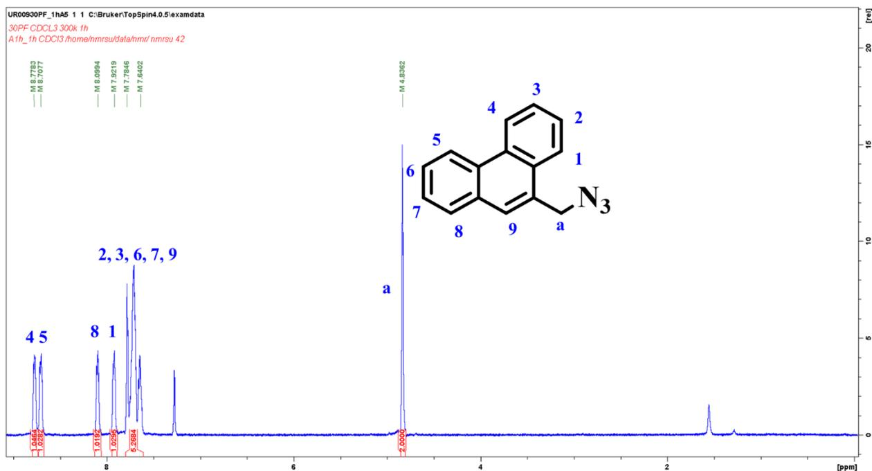
**Figure S3.**  $^1\text{H}$  NMR spectra of compound **4** in  $\text{CDCl}_3$ .
