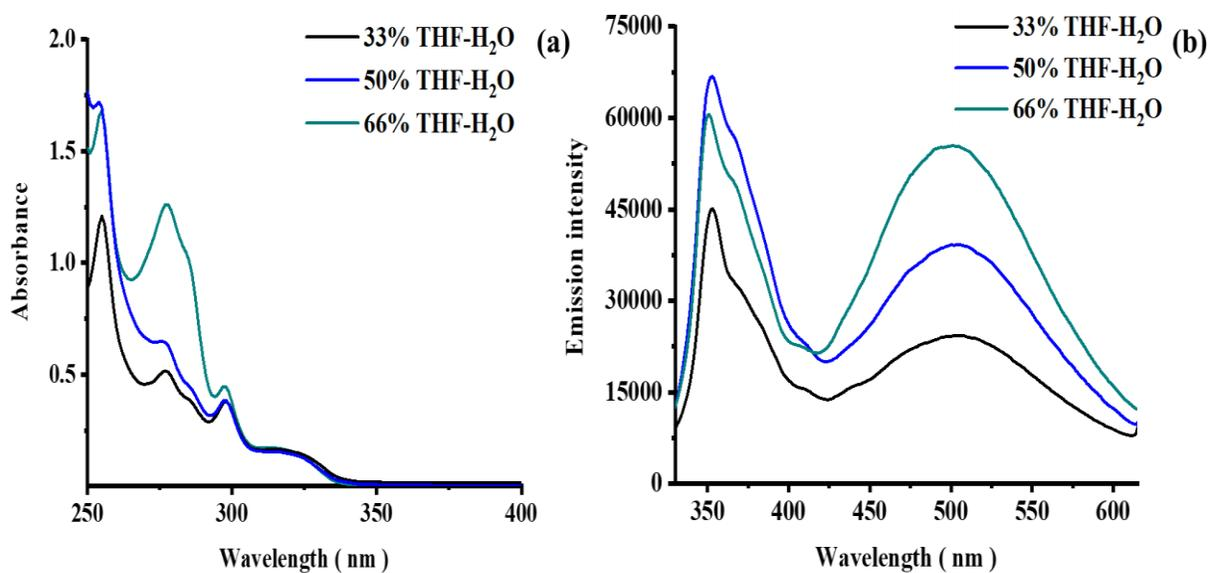
**Figure S12.** (a) Absorption and (b) emission spectra of dyad **8** (5  $\mu\text{M}$ ) in different THF-water mixtures in a B-R buffer (25 mM).
