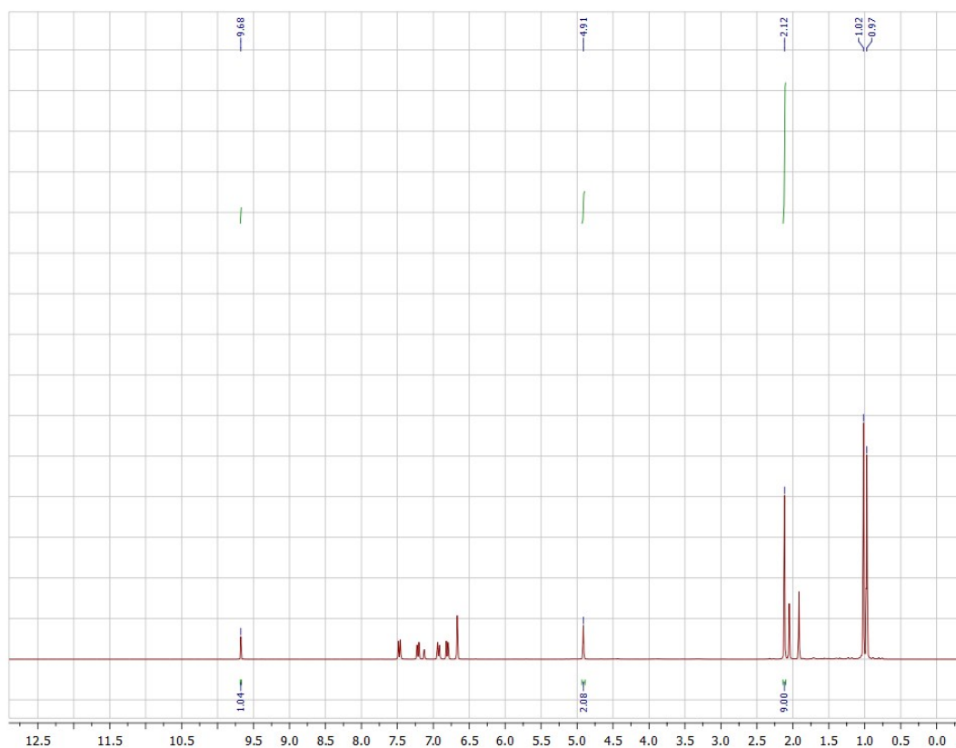
Figure S35. ^1\text{H} NMR spectra for Hydroboration of 4-Methylbenzaldehyde with HBPin in benzene- \text{d}_6 using catalyst (1) loading of 1 mol% for 1 hrs at room temperature.
