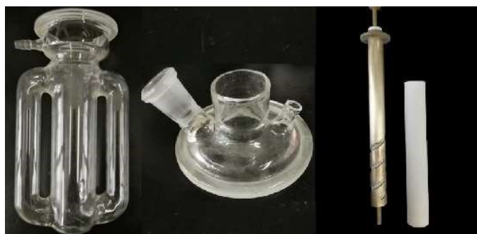
Figure 2. MW loop reactor: loop reactor (left); cover (middle); leaky coaxial antenna and PTFE sleeve (right). The cover is provided with three ports for connection of condenser, antenna insertion, and temperature detection (sampling) respectively. The antenna is centered in the reactor. The sleeve covers the exterior of the antenna to avoid the direct exposure of the antenna to the material.
