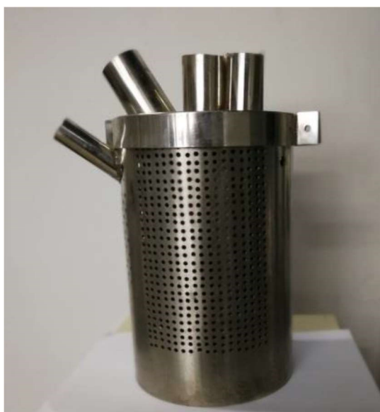
Figure 3. Stainless steel shielding cover
