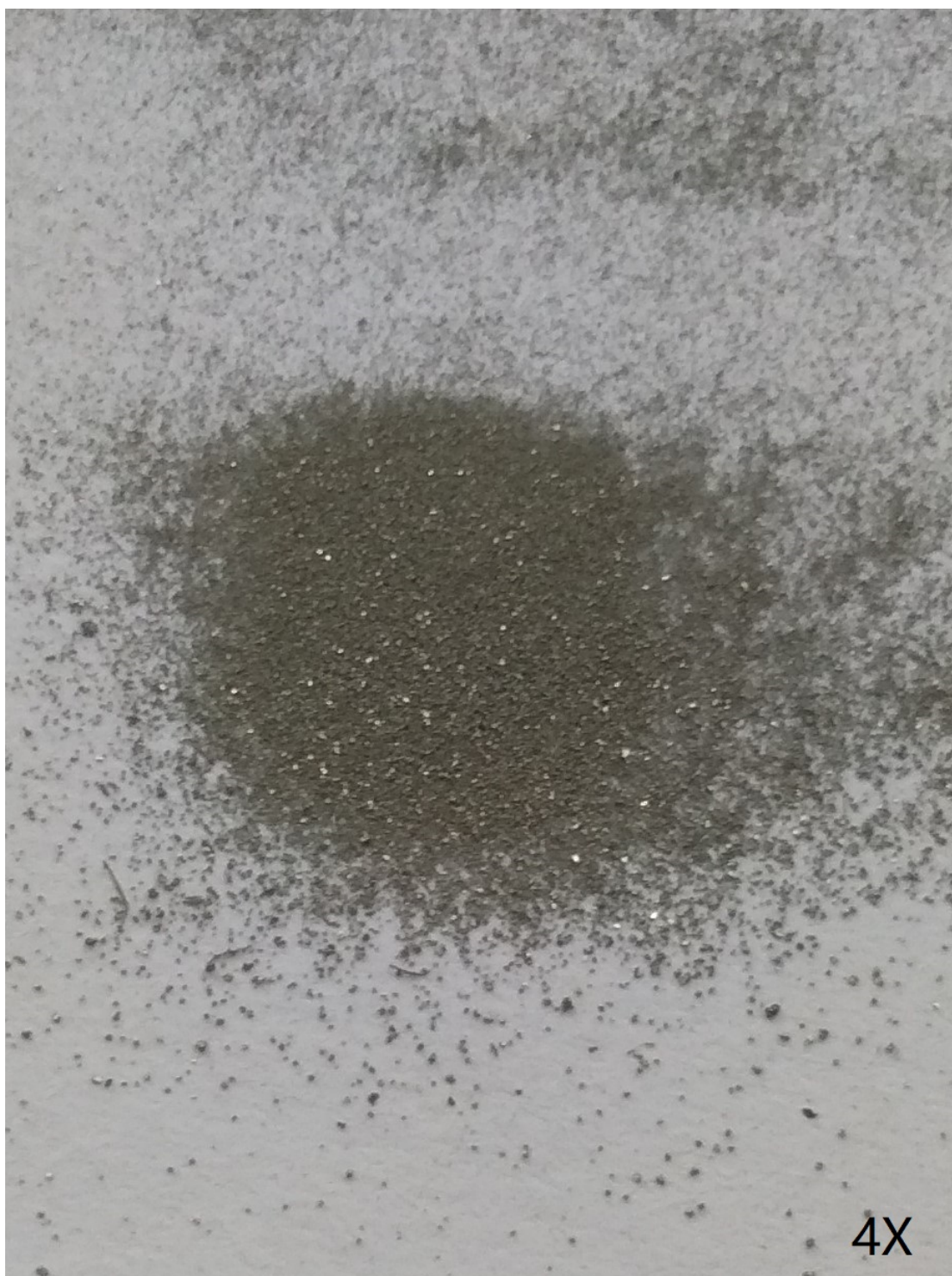
Zn powders after ball-milling, (h) in Fig 1
