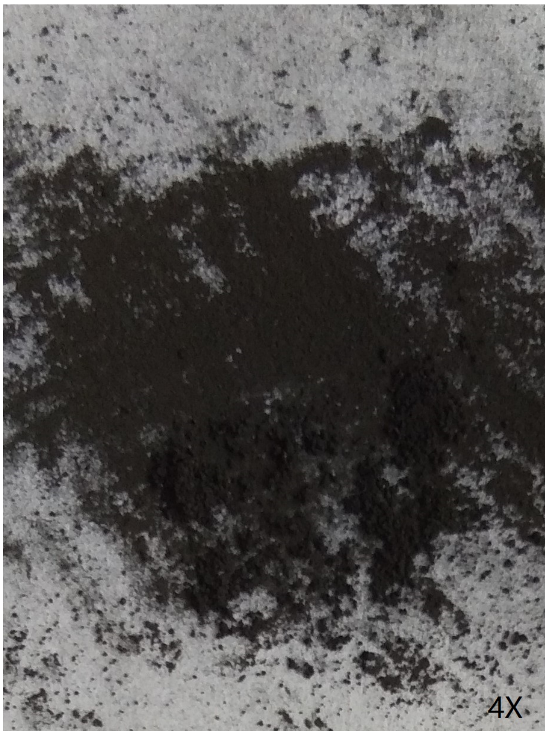
Mn powders after ball-milling, (b) in Fig 1.
