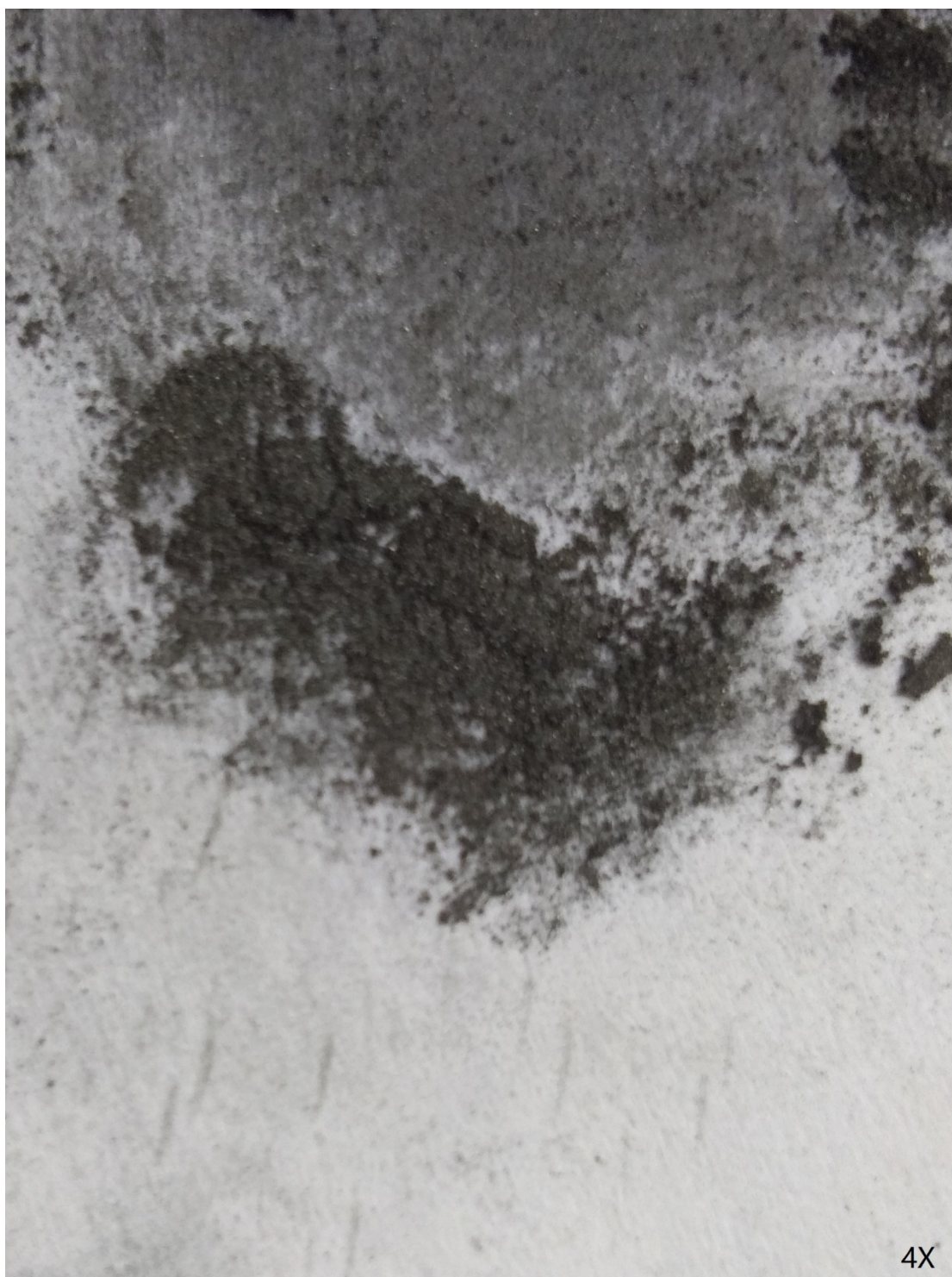
Fe powders after ball-milling, (f) in Fig 1
