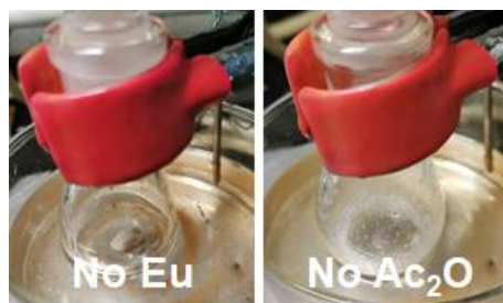
Fig. S9 Photographs of the reaction mixture in control experiments: (left) the reaction mixture of anisole and acetic anhydride; (right) the reaction mixture of anisole and europium(III) triflate.
