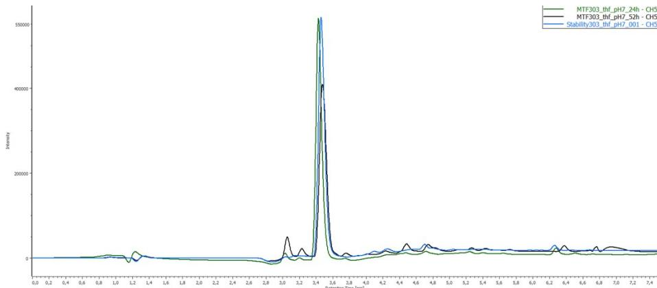
**Stability in cell media (DMEM-PS + FBS).** An aliquot of the 10 mg/mL stock solution of **B1** prepared in THF was taken and incubated in the cell media used in the experiments of cell viability (DMEM-PS + FBS) containing 33% THF to improve solubility. Aliquots were taken and injected for 96 h to the UPLC (*Method B, 254 nm*).
