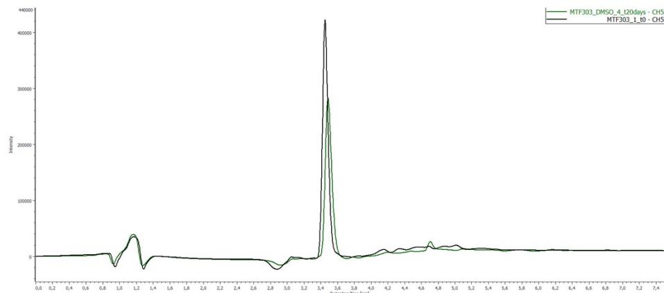
**Stability in THF.** A 10 mg/mL stock solution of **B1** was prepared in THF and incubated at 20°C. Aliquots were taken and injected for 96 h in methanol to the UPLC (*Method B, 254 nm*).
