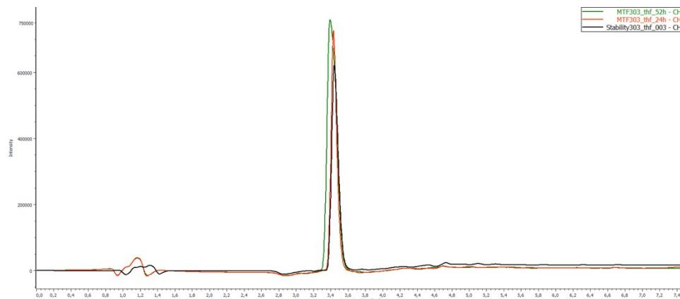
**Stability in 0.1 M phosphate buffer pH 7.0.** An aliquot of the 10 mg/mL stock solution of **B1** prepared in THF was taken and incubated in 0.1 M phosphate buffer pH 7.0 containing 33% THF to improve solubility. Aliquots were taken and injected for 96 h to the UPLC (*Method B, 254 nm*).
