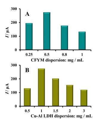
Fig. S1. Optimization of parameters influencing the preparation of Cu-Al LDH/CFYM/GPGE based on DCF oxidation response ([DCF] =  $47.6 \, \mu M$ : (A) influence of concentration of CFYM, and (B) influence of concentration of Cu-Al LDH dispersion.
