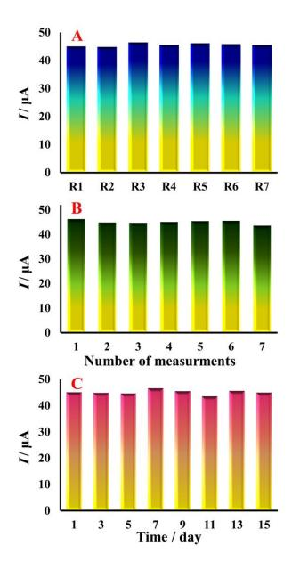
**Fig. S2**. DPV current response of (A) reconstruction, (B) repeatability, and (C) storage stability on the Cu-Al LDH/CFYM/GPGE sensor in PBS solution (pH = 7.0) containing 47.6  $\mu$ M DCF.
