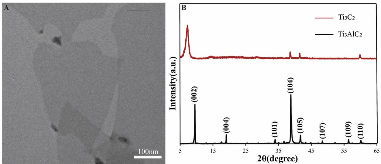
Fig. s7 The TEM image (A) and XRD patterns (B) of  $Ti_3C_2$  and  $Ti_3AlC_2$
