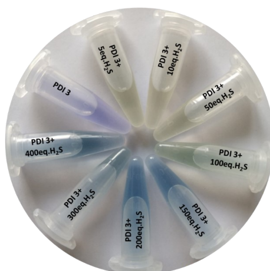
Figure S12: Colour change photos of PDI 3 with gradual addition of H 2 S (naked eye) in 30% urine sample.
