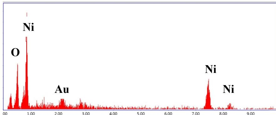
**Figure S-2.** EDX spectra of Ni-NiO nanoparticles.
