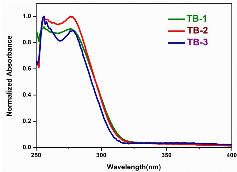
Figure S19. UV-Vis Absorption spectra of TBs.
