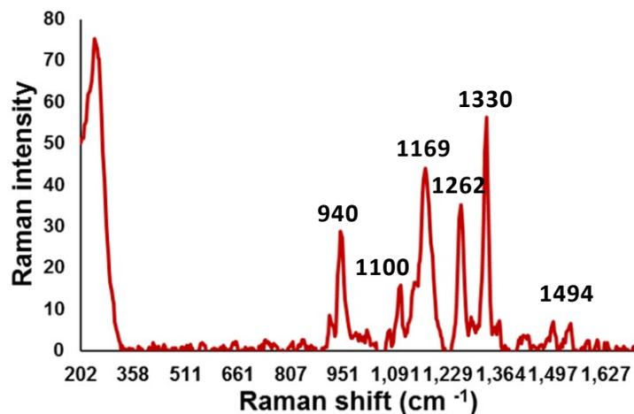
**Figure S16.** SERS Spectrum of SARS-CoV-2 Spike protein excited under 633 nm laser.
