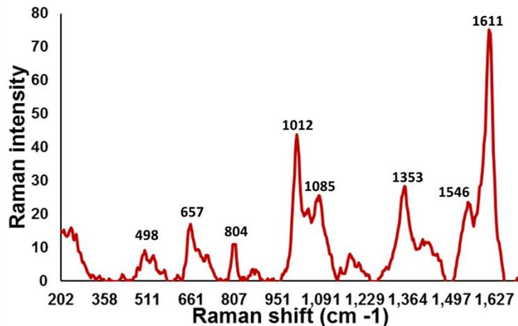
**Figure S14.** SERS Spectrum of TB-3 excited under 633 nm laser.
