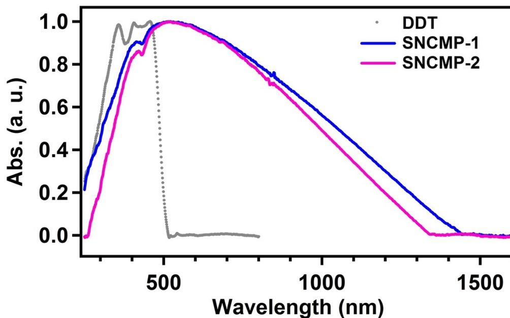
**Figure S4.** The normalized solid state UV-Vis spectra of SNCMP-1 and SNCMP-2.
