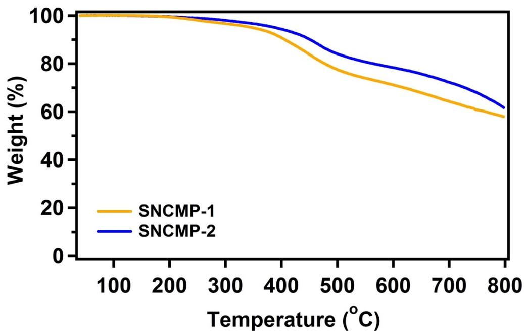
Figure S6. TGA curves of SNCMP-1 and SNCMP-2.
