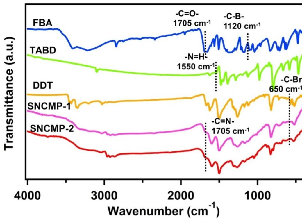
Figure S1. FT-IR spectra of SNCMP-1 and SNCMP-2.
