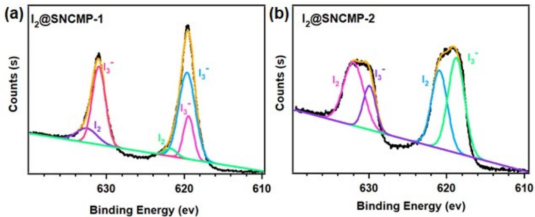
**Figure S10.** XPS spectra for I3d3 and I5d5 in the (a)  $I_2@SNCMP-1$  and (b)  $I_2@SNCMP-2$ .
