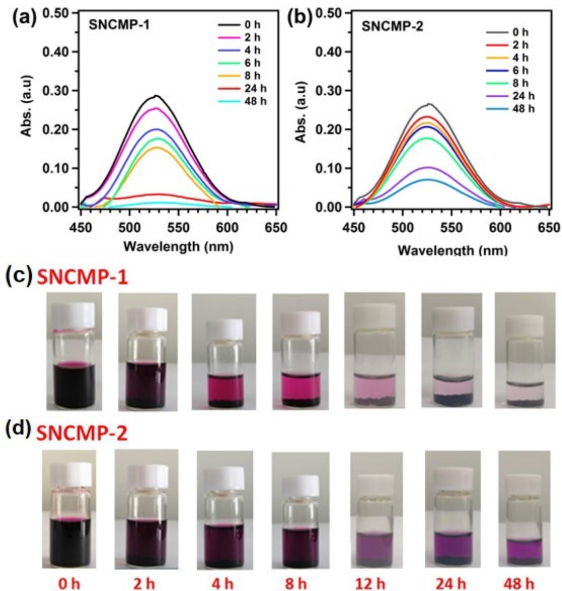
**Figure S13.** (a-b) the UV-Vis spectra upon immersion of 30 mg SNCMPs in cyclohexane solution of I<sub>2</sub> (6 mg ml<sup>-1</sup>). All experiments were performed at ambient temperature and pressure. (c-d) Photographs show the adsorption rates of SNCMPs at various time intervals. The weight of the adsorbent (30 mg) immersed in a cyclohexane solution of I<sub>2</sub> (6 mg mL<sup>-1</sup>, 5 mL) at room temperature.
