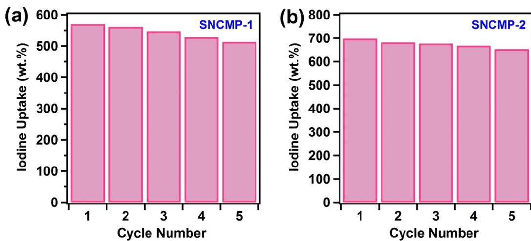
**Figure S12.** Reusabilities of the (a) SNCMP-1 and (b) SNCMP-2 polymers for iodine adsorption by vapor sublimation.
