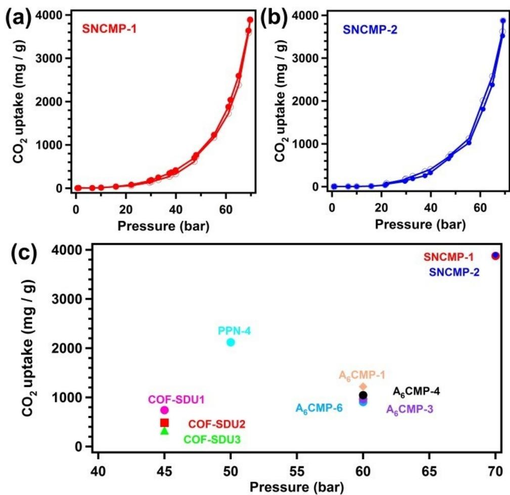
**Figure S15.** CO<sub>2</sub> adsorption isotherms of (a) SNCMP-1 and (b) SNCMP-2 collected at 70 bar and 323 K, (c) the summary of CO<sub>2</sub> capture of polymers at high pressure.
