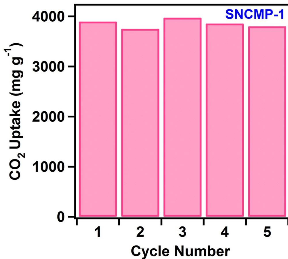
Figure S16 Carbon dioxide adsorption cycle of SNCMP-1.
