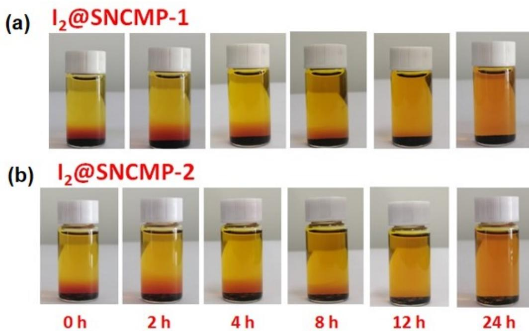
**Figure S11.** Photographs showing progress of the iodine release from (a)  $I_2@SNCMP@1$  and (b)  $I_2@SNCMP@2$ , when the containing iodine polymer networks were immersed in ethanol.
