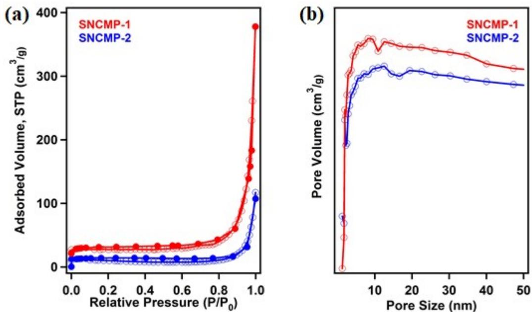
**Figure S7.** (a) Nitrogen sorption curves and (b) pore size distribution curves of SNCMP-1 and SNCMP-2.
