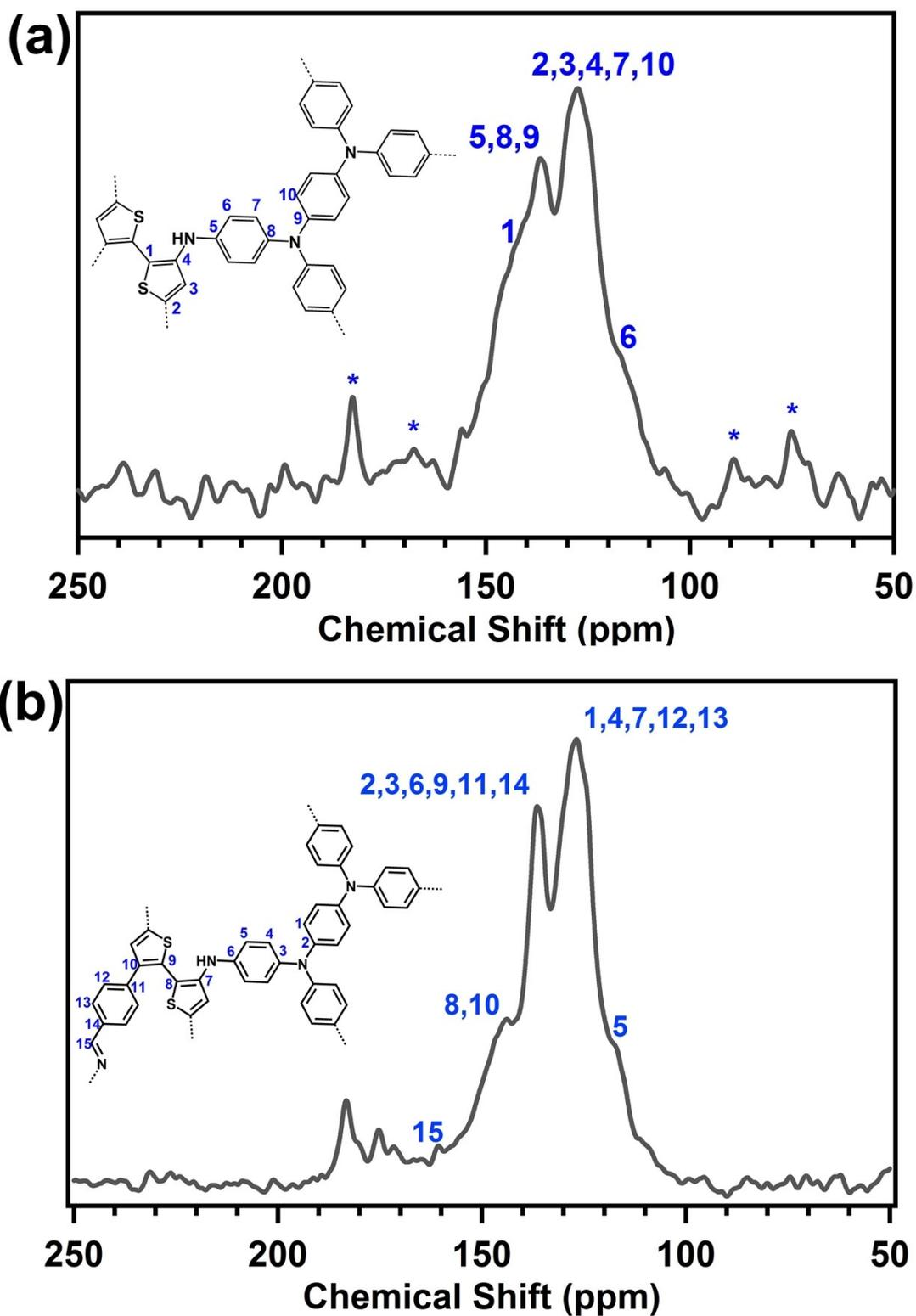
Figure S2. The solid-state  $^{13}\text{C}$  CP-MAS NMR of (a) SNCMP-1 and (b) SNCMP-2.
