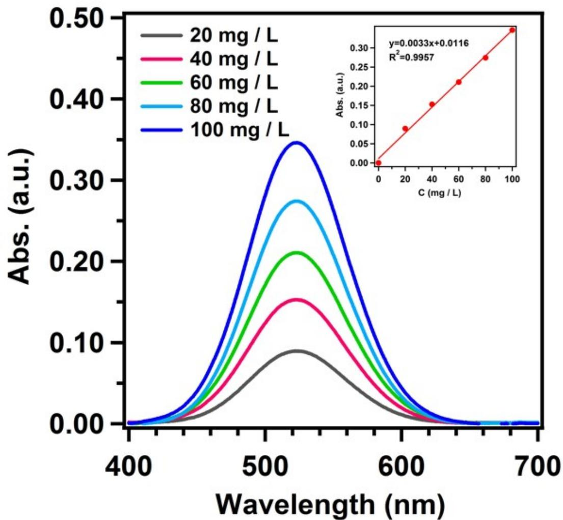
**Figure S14.** The standard curve of iodine in cyclohexane solution (Inset is the fitting curve of Abs value vs concentration of iodine in cyclohexane solution, the value of  $R^2$  indicated that the curve with the relatively good linearity satisfies Lambert-Beer Law. The iodine adsorption capacity of SNCMPs was calculated according to the standard curve).
