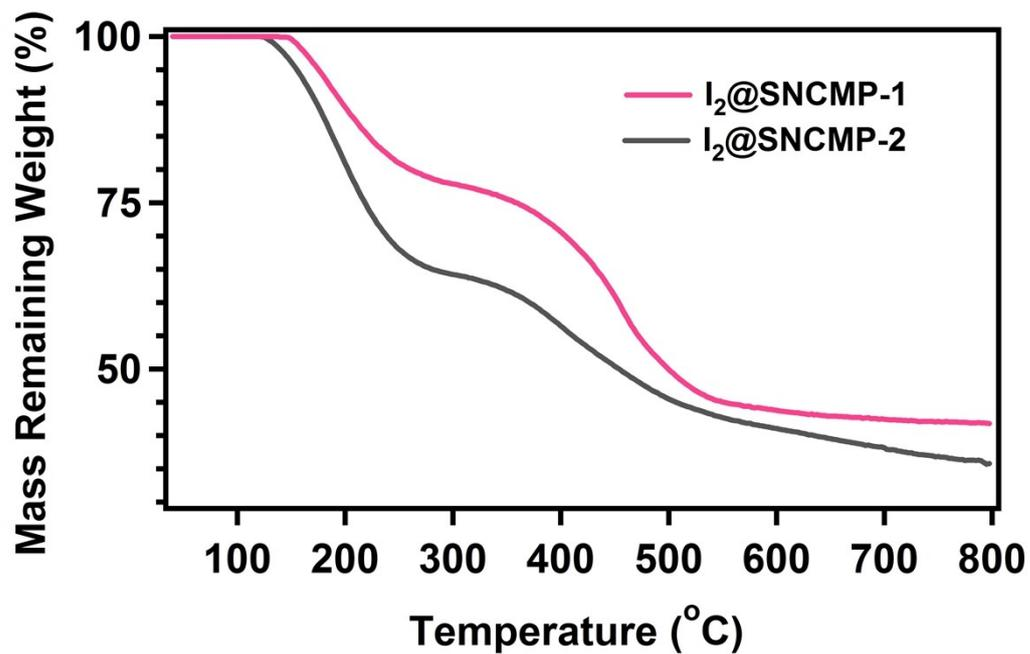
Figure S8. TGA curves of I<sub>2</sub>@SNCMP-1 and I<sub>2</sub>@SNCMP-2.
