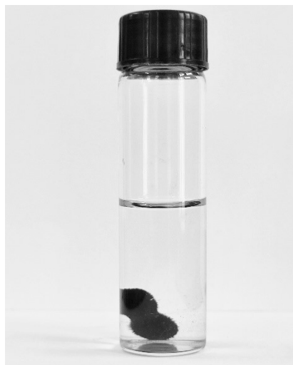
Fig. S5. (a) Reaction mixture of Anhydride, Methanol and \text{Fe}_3\text{O}_4@\text{mQD} NPs under stirring with magnetic bar (b) reaction mixture when magnetic stirring is stopped and the catalyst sticks to the magnetic needle.
