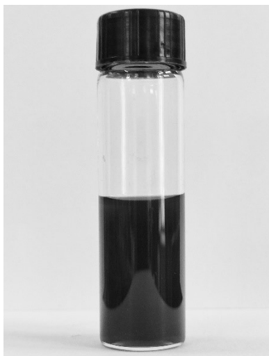
Fig. S5. (a) Reaction mixture of Anhydride, Methanol and \text{Fe}_3\text{O}_4@\text{mQD} NPs under stirring with magnetic bar (b) reaction mixture when magnetic stirring is stopped and the catalyst sticks to the magnetic needle.
