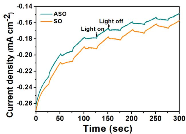
**Figure S2.** Photo response of the discharge voltage in a photo-assisted Li–O<sub>2</sub> battery with a current density of 100 mA g<sup>-1</sup> when illumination is switched from "on" to "off".
