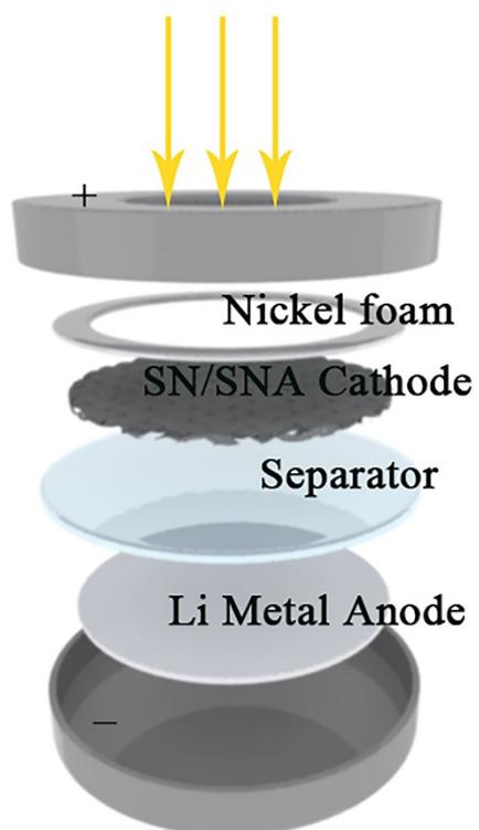
**Figure S3.** Schematic configuration diagram of light-assisted Li-O<sub>2</sub> battery.
