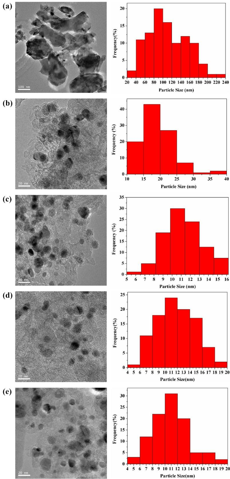
**Figure S1.** HR-TEM images (Left) and Particle size distribution statistics (right) of the as-prepared (a) Co-N/C-800-1, (b) Co-N/C-800-2, (c) Co-N/C-800, (d) Co-N/C-800-10, (e) Co-N/C-800-45.
