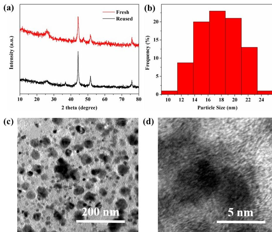
**Figure S3** (a) XRD spectra of the reused Co-N/C-800 catalyst; (b) Particle size distribution statistics of deactivation Co-N/C-800 catalyst; TEM images of partial deactivation Co-N/C-800 catalyst (c) at 200 nm, (d) at 5 nm.
