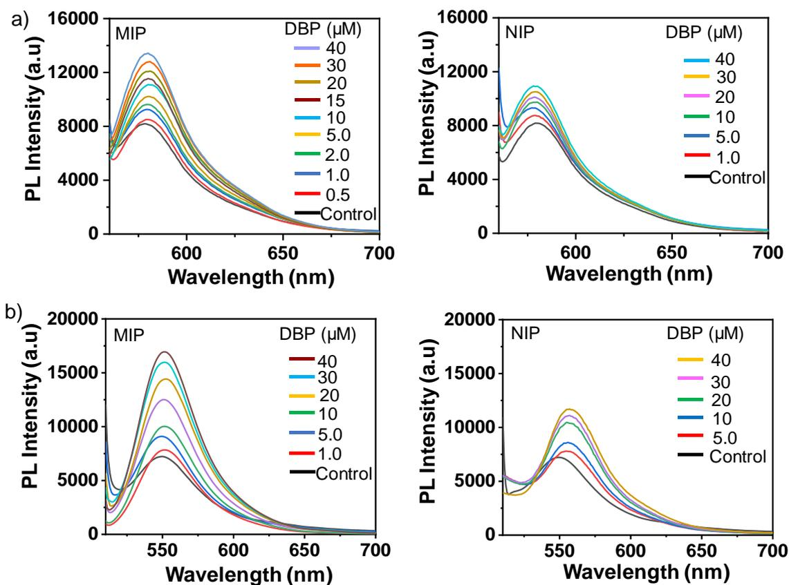
**Figure S5.** Fluorescence ‘turn on’ response using rhodamine B (emission maxima = 580 nm) (a) and rhodamine 6G (emission maxima = 550 nm) (b). The selectivity as well as sensitivity is not up to the mark with these dyes.
