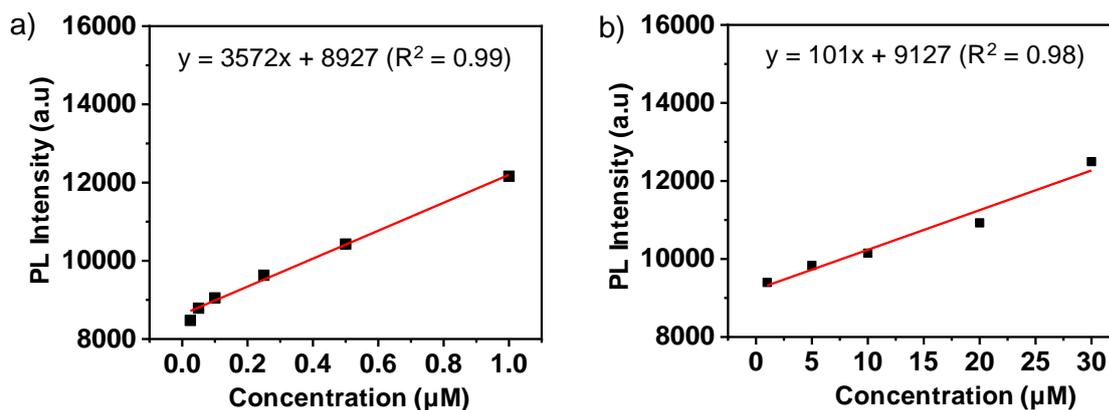
**Figure S3.** Linear calibration curves of fluorescence intensity with the variation of DBP concentration for MIP (a) and NIP (b). Limit of detection (LOD) =  $3\sigma/K$ , where  $\sigma$  is the standard deviation of blank measurement, K is the slope of the linear curve. LOD calculated for MIP and NIP appears as 24 nM and 3.5  $\mu\text{M}$ , respectively.
