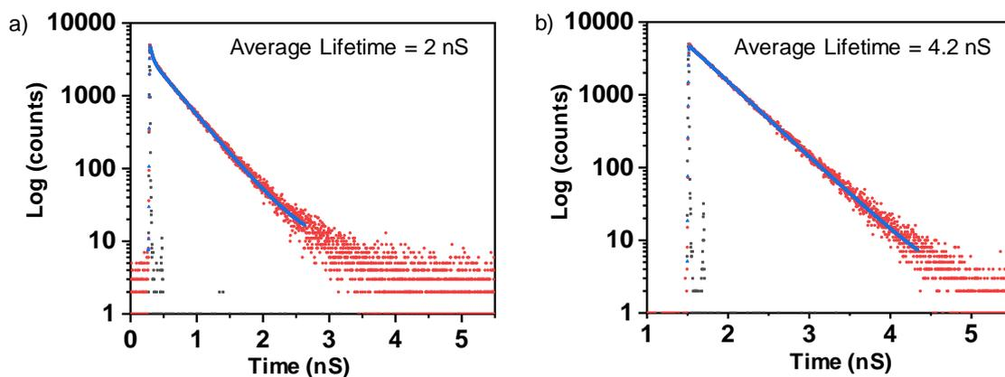
**Figure S7.** Fluorescence lifetime decay curve of fluorescein after binding with MIP (a) and after release via DBP addition (b). The fluorescence lifetime increases in presence of DBP due to inhibition of non-radiative energy transfer.
