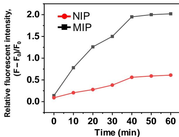
**Figure S8.** Fluorescence ‘turn on’ kinetic by addition of DBP to MIP/NIP-fluorescein. This result shows that the dye displacement maximises around 60 min of contact time with DBP.
