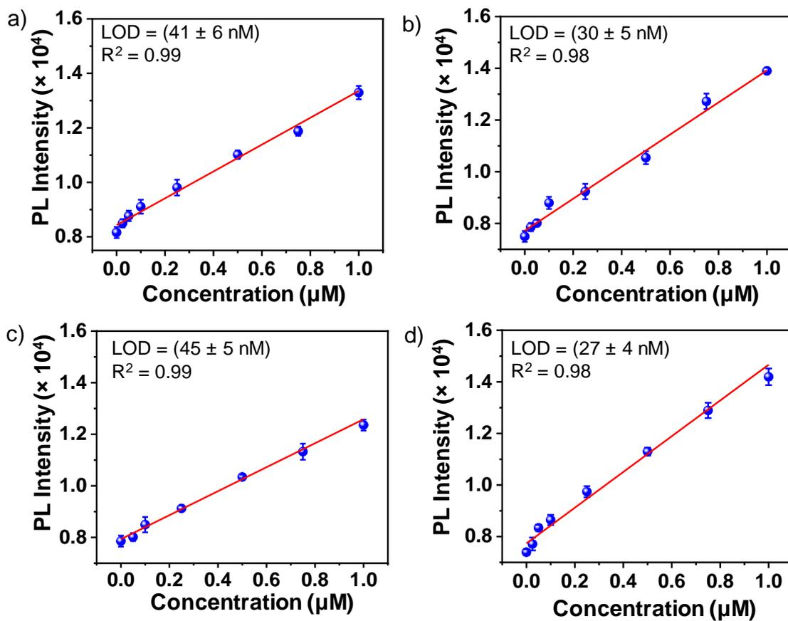
**Figure S9.** Linear fluorescence increment calibration curve and LOD values for DBP detection with MIP in different real water matrices. a) tap water, b) lake water, c) river water and d) waste water. All experiments were performed at 25 °C and error bar represents three independent experiment.
