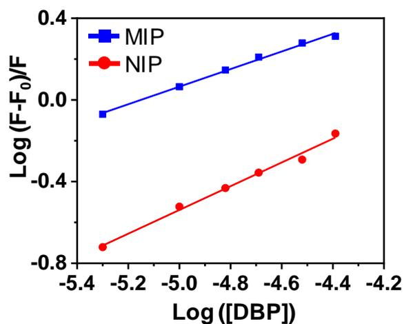
**Figure S4.** Calculation of binding constant between MIP/NIP and DBP by plotting  $\log \{(F - F_0)/F\}$  vs  $\log ([\text{DBP}])$  following the equation:  $\log \{(F - F_0)/F\} = n \log ([\text{DBP}]/K_D)$ , where  $F_0$  and  $F$  are the fluorescence intensity before and after addition of DBP. The binding constant ( $K_B = 1/K_D$  ( $\text{M}^{-1}$ )) and values appears as  $8.2 \times 10^4$  and  $3.5 \times 10^3$  for MIP and NIP, respectively.
