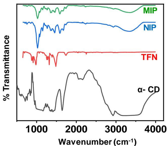
**Figure S1.** FTIR spectra of MIP, NIP, TFN, and  $\alpha$ -CD showing the formation of the polymer nanocomposite. C–F stretching band around  $1455\text{ cm}^{-1}$  appears for MIP and NIP.
