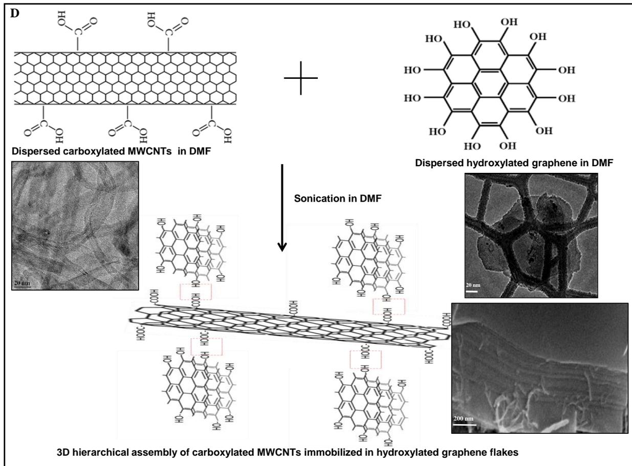
Fig S1: Schematic representation of the preparation methods for (A) 0D, (B) 1D, (C) 2D and (D) hybrid hierarchical functional nanofillers.
