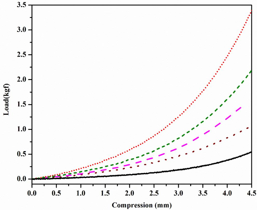
Fig S4: The comparative flexural strength of PVA hydrogel (black thick line) and 0.5 weight percentages of carbon nanoparticles (brown dotted line), carbon nanotubes (green short dashed line), graphene (magenta dashed line) and CNT immobilized graphene flakes (red short dotted line) were represented.
