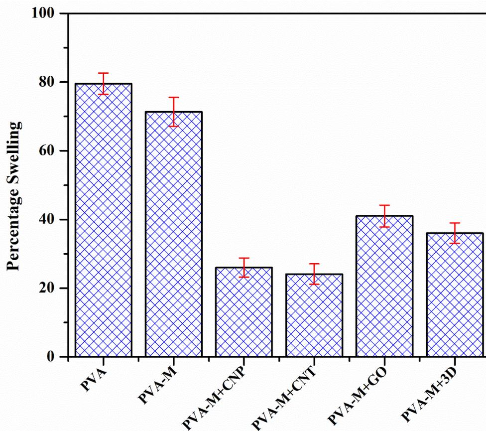
Fig S3: The extent of swelling of PVA, PVA-melamine (PVA-M) hybrid network hydrogel, PVA-melamine nanocomposite gels with 0.5 weight percentages of carbon nanotubes (PVA-M+CNT), carbon nanoparticles (PVA-M+CNPs), graphene (PVA-M+GO) and CNTs embedded into graphene flakes (PVA-M+3D) are represented graphically.
