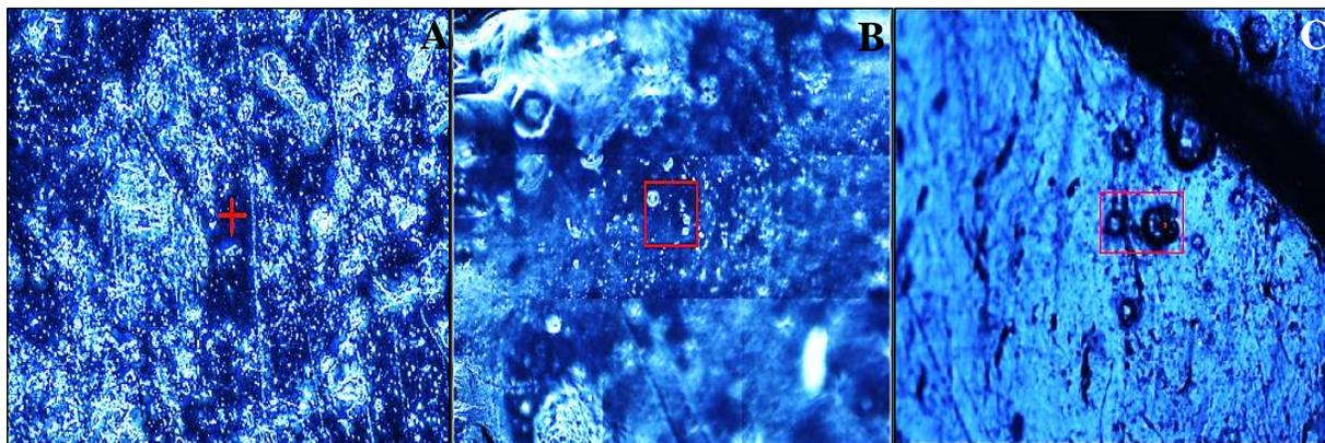
Fig S7: The optical microscopic images using 5X objective of nanocomposite hydrogel samples have been displayed where the loading of functionalized multiwalled carbon nanotubes were varied as (A) 0.25, (B) 0.5 and (C) 1.0 weight percentages.
