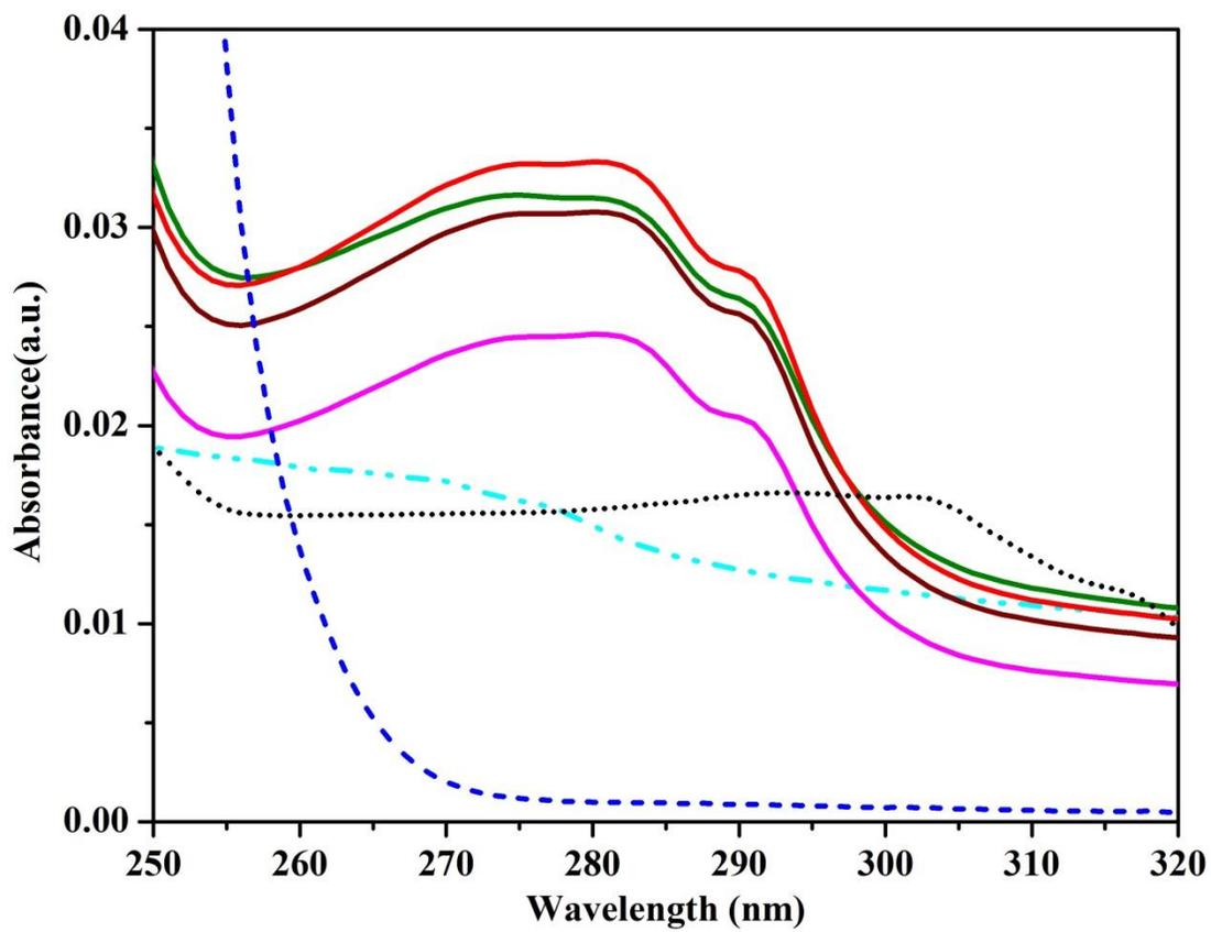
Fig S5: The UV absorption spectra of PBS enzyme solution (black dotted line), PVA solution (sky blue dashed dot line) and melamine solution (deep blue dashed line) are illustrated in the figure. The UV absorption of enzymatically degraded solution of the nanocomposite hydrogels of 0.5 weight percentages of carbon nanoparticles (brown), carbon nanotubes (green), graphene (magenta) and CNT immobilized graphene flakes (red) after 06 days were represented.
