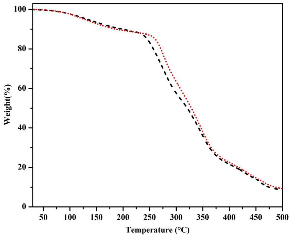
Fig S2: Thermogravimetric (TGA) analysis result of PVA hydrogel (black dashed line) and PVA-melamine (red dotted line) hybrid crosslinked hydrogel.
