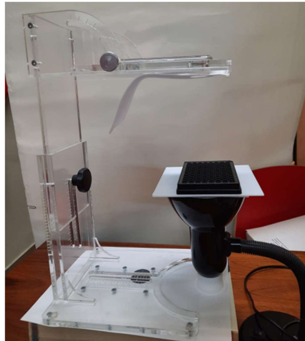
Figure S. 2. The proposed setup consisted of a desktop lamp as a light source, and a methacrylate stand to place the smartphone. A white diffusive material is placed between the LED bulb and the samples.
