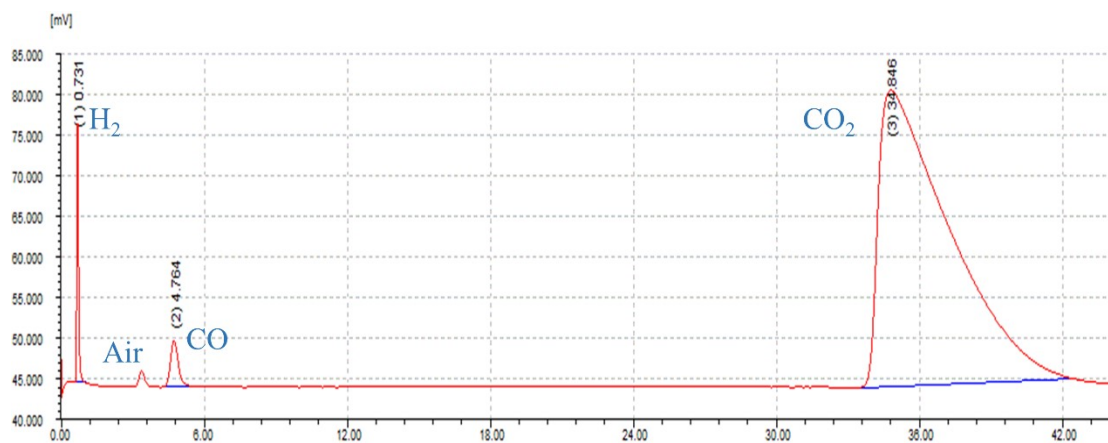
Fig. S3. Gas chromatography of product gases.
