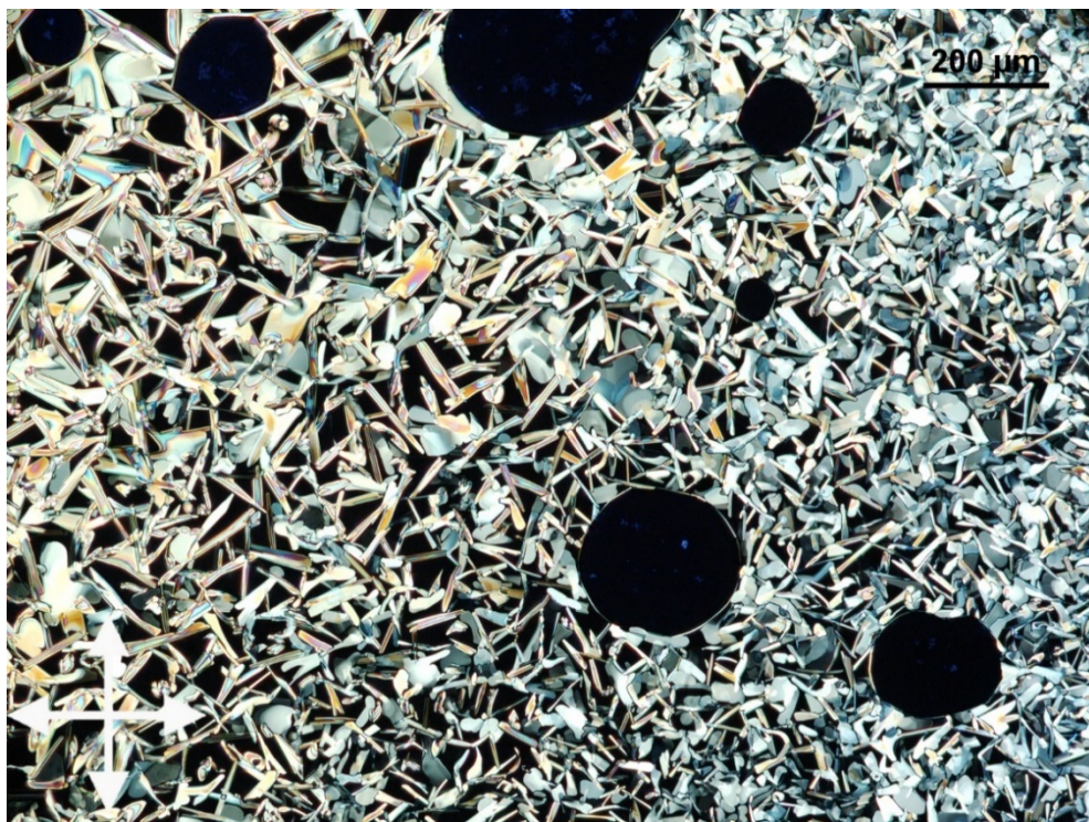
Figure S10. Polarized optical microscopy image of the \text{PtCl}_2 complex at 140 °C after cooling from the isotropic phase (crossed polarisers are represented by the white cross in the corner).
