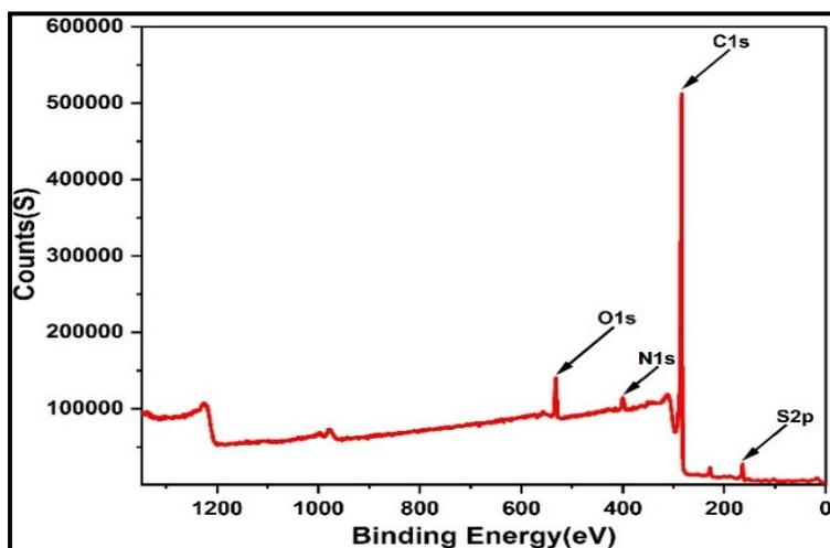
**Fig. S-2** XPS Survey spectrum of g-SFCSSs.**Table S-1** Elemental peak table of XPS analysis of g-SFCSSs.
