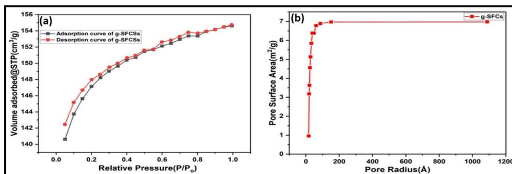
**Fig. S-4** (a) Nitrogen adsorption – desorption isotherm of g-SFCs, (b) Pore size distribution of g-SFCs
