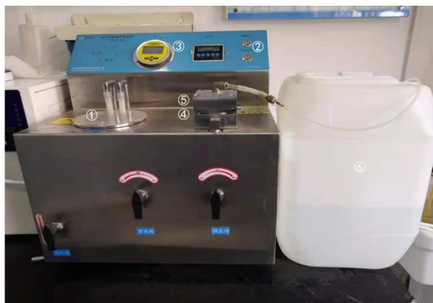
① Storage tank full of simulated natural seawater; ② Pump; ③ Pressure indicator; ④ Jute-TMC-PAO fabric; ⑤ Diaphragm clamping; ⑥ Recovery tank
