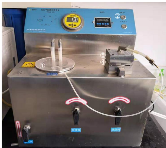
① Storage tank; ② Pump; ③ Pressure indicator; ④ Jute-TMC-PAO carpet; ⑤ Diaphragm clamping.
