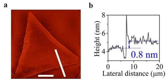
Figure S1. (a) AFM image of the prepared sample. (b) Height profiles corresponding to the solid line in a. The thickness of  $\sim 0.8$  nm confirms that the prepared sample is monolayer.
