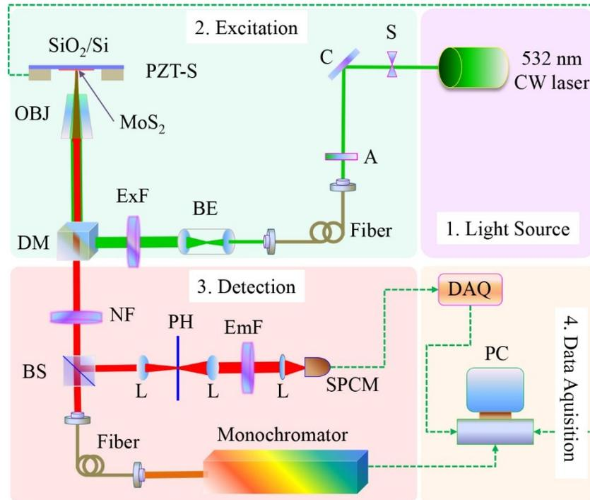
Figure S2. Schematic diagram of the optical setup. S: shutter; C: beam combiner; A: attenuator; BE: beam expander; ExF: excitation filter; DM: dichroic mirror; OBJ: objective; PZT-S: piezo-electric translation nano-stage; NF: notch filter; BS: beam splitter; L: lens; PH: pinhole; EmF: emission filter; SPCM: single-photon counting modular; DAQ: data acquisition card; PC: personal computer.
