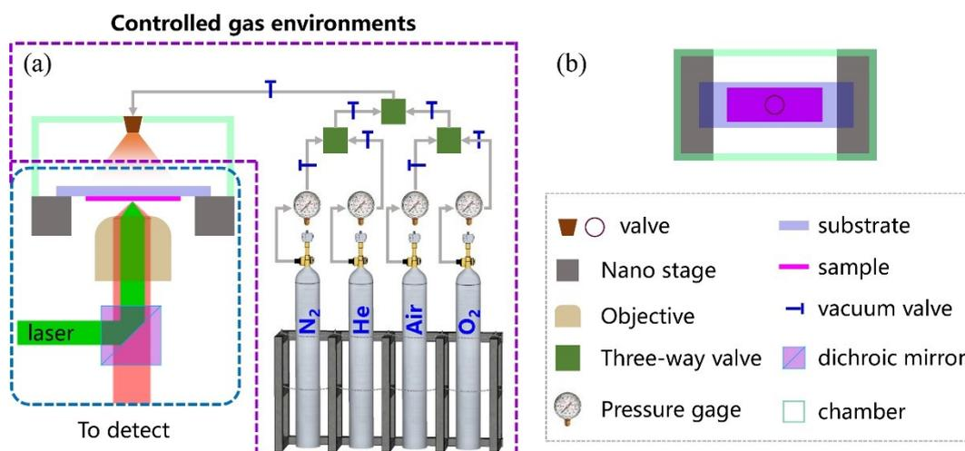
Figure S3. Schematic illustration of the controlled gas environments. (a) Gases were blowing from the backside of the substrate; the bottom of the chamber was opened. The blowing rate of gases was kept constant at 1 L/min. PL quenching processes were performed by just stopping to blow N<sub>2</sub>, rather than sweeping the dry air gases. (b) Top view of the setup.
