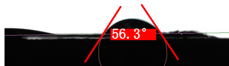
Figure S2. Contact angle measurements of (a)Mo-Ni 3 S 2 QDs (b)Ni-LDH@Mo-Ni 3 S 2 , (c)Mo-Ni 3 S 2 and (d) Ni-OFG.
