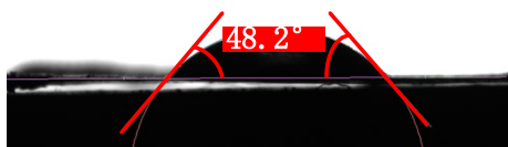
Figure S2. Contact angle measurements of (a)Mo-Ni 3 S 2 QDs (b)Ni-LDH@Mo-Ni 3 S 2 , (c)Mo-Ni 3 S 2 and (d) Ni-OFG.
