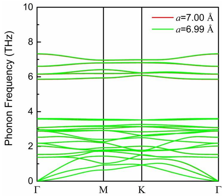
**Figure S7.** Phonon dispersion for FM-CrI<sub>3</sub> when lattice constant  $a$  is 7.00 and 6.99 Å, respectively.
