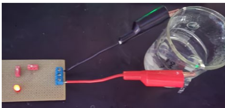
Fig. S7 The photographic image of the ASC device lighting up one LED.
