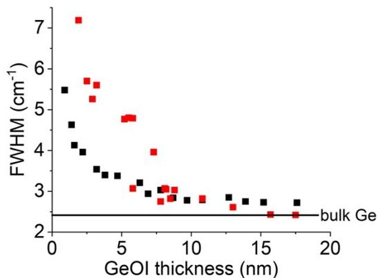
Fig. 1. Dependence of the LO phonon Raman band FWHM on  $T_{\text{GeOI}}$  for uncoated (black squares) and  $\text{Al}_2\text{O}_3$ -coated (red squares) GeOI.
