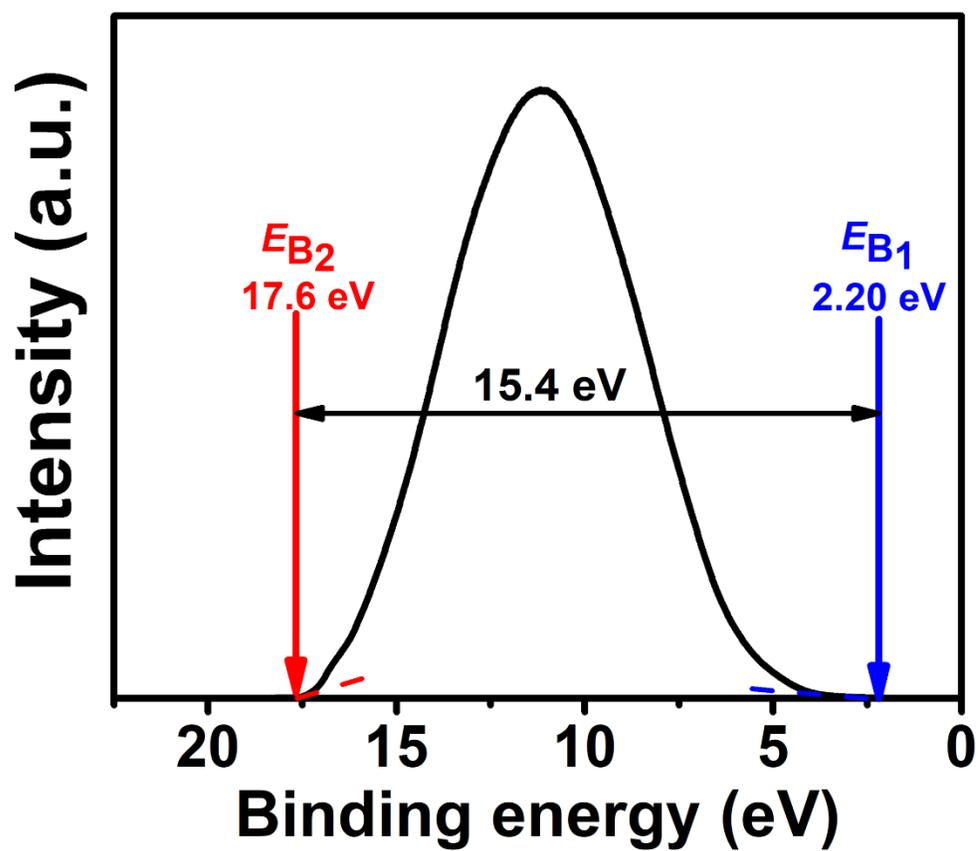
**Fig. S4** UPS spectrum of NGODs. The electron onset binding energy values,  $E_{B1}$  and  $E_{B2}$ , were determined from the intercepts of the extrapolated tangent lines on the abscissa at low and high binding energies, respectively. The UPS width constituted the difference between  $E_{B1}$  and  $E_{B2}$ . The spectrum was obtained under He I light irradiation at 21.2 eV.
