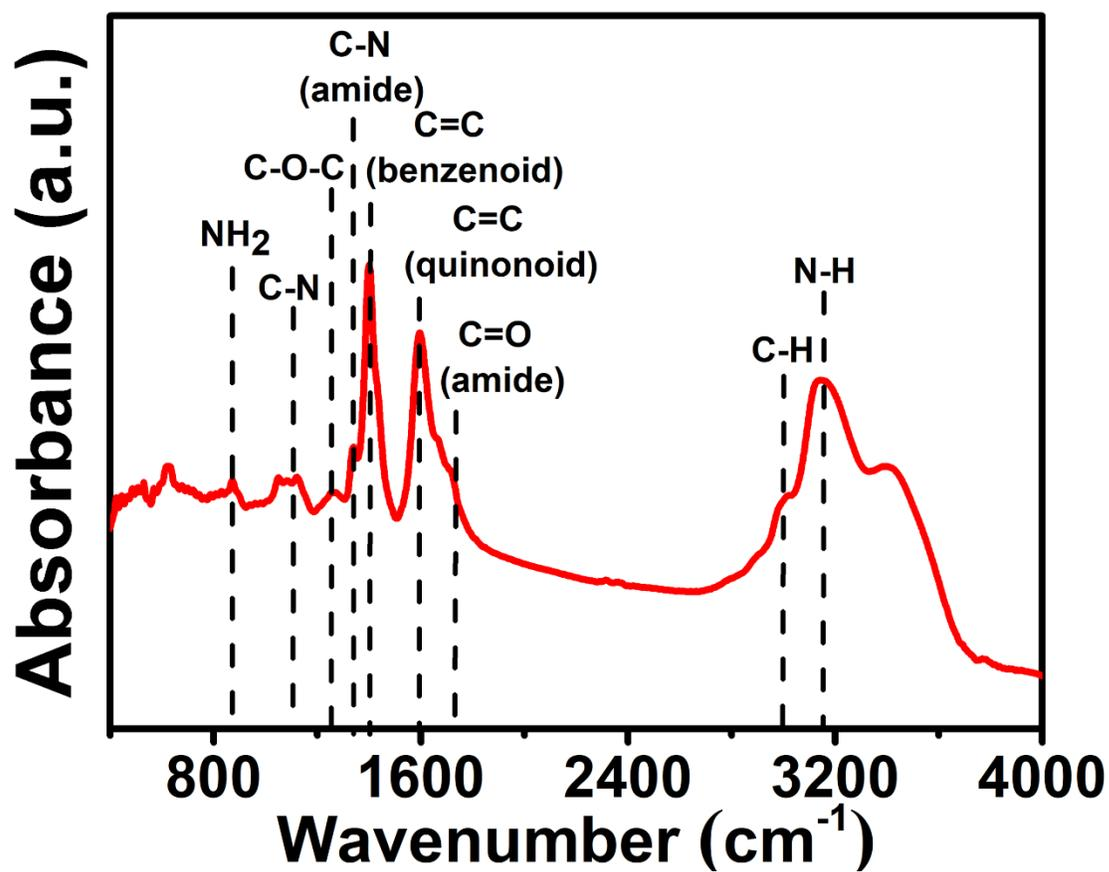
Fig. S3 FTIR absorption spectrum of NGODs.
